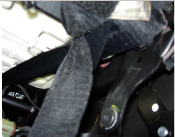
Step 16. Driver & Passenger Top/DT&PT: Route each of the long hook Velcro™ under the back edge of the seat and around the outside support wire, the same area the plastic clip connected to. Take up the slack again as in Step 15, then reach under the seat and take up the slack in the Velcro™ by pulling it forward and connect as shown in Step 17. Then press the seat cover with one hand to the seat while taking up the slack in the Velcro™ with the other hand.
