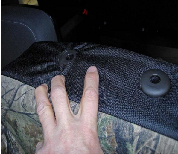
Step 13. Driver & Passenger Top/DT&PT: Tuck the seat cover under the plastic for the headrests, starting on the push button side.
