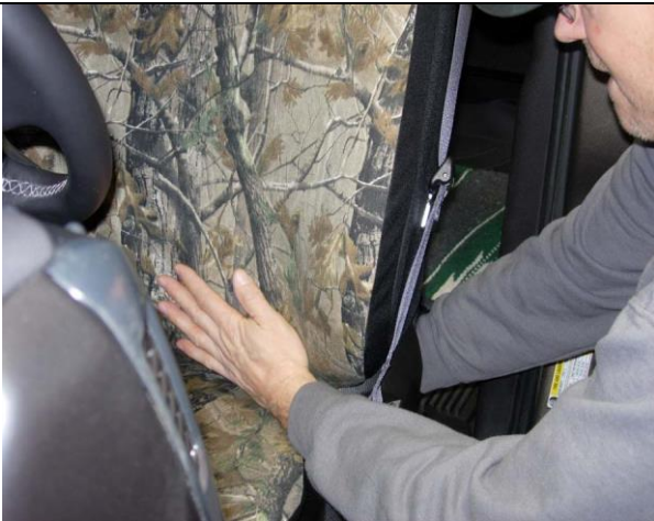
Step 15. Driver & Passenger Top/DT&PT: While pulling on the seat cover from behind, right where the Velcro™ is sewn on, slide one hand down the front side of the seat in a smoothing action taking up the slack. Make sure you're backrest are positioned slightly forward from normal. When the seat cover is fully installed, recline the backrests to the normal positions, it'll help tighten the front side even more.
