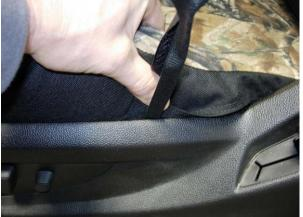
Step 8. Driver & Passenger Bottom/DB&PB: Likewise with the left and right side Velcro<sup>™</sup>, fold them in half lengthwise. Push the outside edge Velcro<sup>™</sup> straight down where shown.
