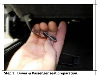
Feel under the back edge of the seat on each side for the elastic straps. They are connected to support wires under the seat with the plastic clips shown in the picture. They're fairly difficult to remove. Pry the plastic clip open while pushing it forward. I used my fingers to pry it open, but you may opt for a tool of
