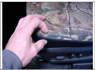
Step 5. Driver & Passenger Bottom/DB&PB: Work the fabric from the seam inside the seat cover outwards, or from forefinger to thumb.
