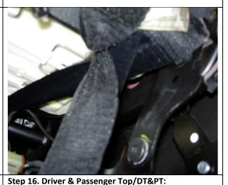
Route each of the long hook Velcro™ under the back edge of the seat and around the outside support wire, the same area the that plastic clip connected to. Take up the slack again as in Step 15, then reach under the seat and take up the slack in the Velcro™ by pulling it forward and connect as shown in Step 17. It's helpful to press the seat cover with one hand to the seat while taking up the slack in the Velcro™ with the other hand.
