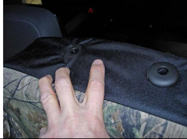
Step 13. Driver & Passenger Top/DT&PT: Tuck the seat cover under the plastic for the headrests, starting on the push button side.
