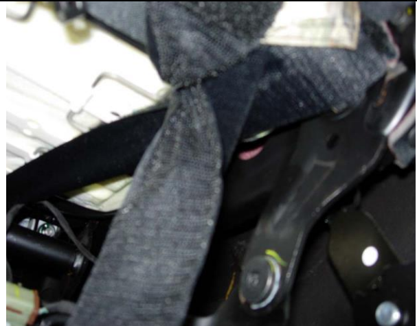
Step 16. Driver & Passenger Top/DT&PT: Route each of the long hook Velcro™ under the back edge of the seat and around the outside support wire, the same area the plastic clip connected to. Take up the slack again as in Step 15, then reach under the seat and take up the slack in the Velcro™ by pulling it forward and connect as shown in Step 17. It's helpful to press the seat cover with one hand to the seat while taking up the slack in the Velcro™ with the other hand.
