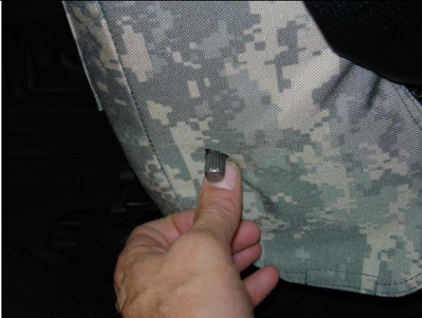
Step 21. Driver & Passenger Tops/DT&PT: Position the hole for the recline lever and press it back onto the seat.
