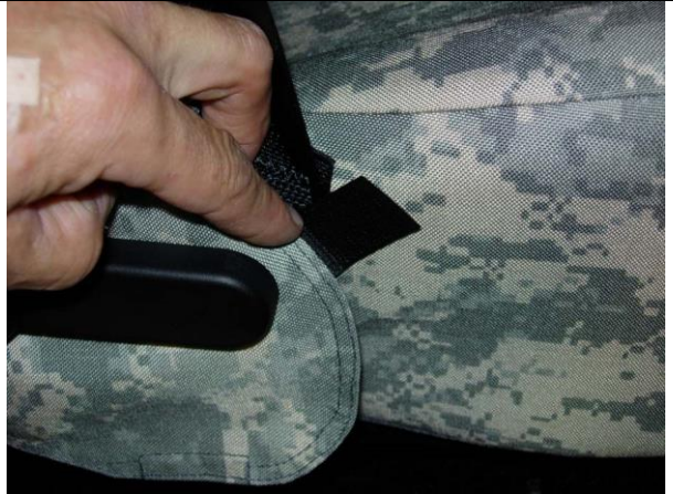
Step 22. Driver & Passenger Tops/DT&PT: Fold this small side hook Velcro™ around the backside and connect it to the carpet on the backside. 2016 does not fasten this way, see Step 23.
