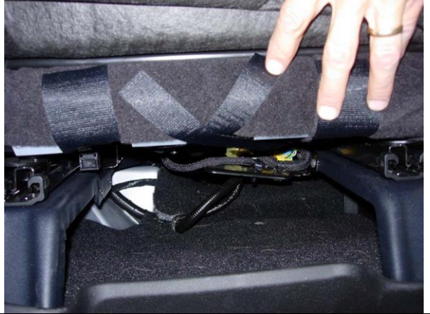
Step 14. Driver & Passenger Bottoms/DB&PB: The side Velcro™ should be fastened in an "X" pattern.
