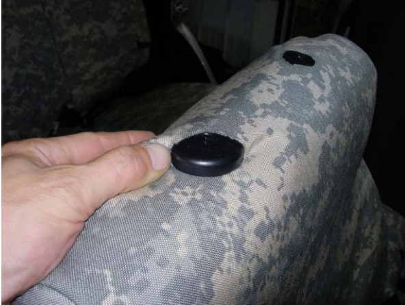
Step 17. Driver & Passenger Tops/DT&PT: Tuck the fabric under the plastic for the headrests.
