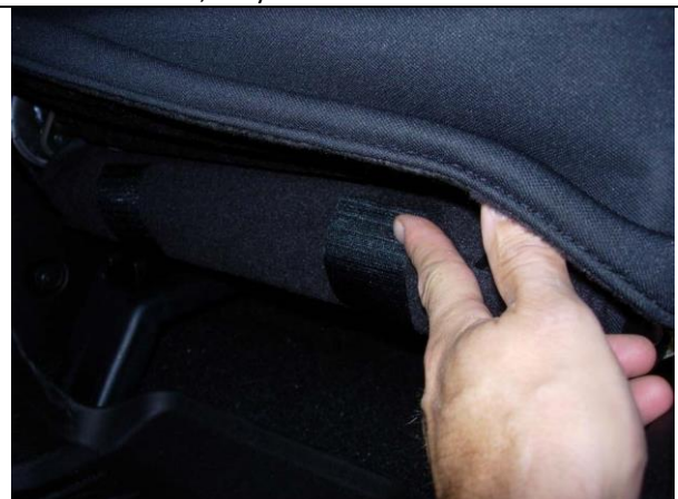
Step 10. Driver & Passenger Bottoms/DB&PB: Connect them to the carpet on the back edge, or if no carpet exists connect them to the loop Velcro™ sewn on the back edge.
