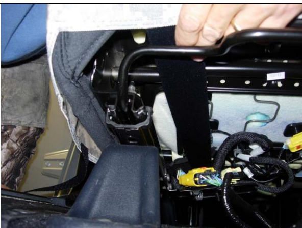
Step 9. Driver & Passenger Bottoms/DB&PB: Route the under the knee Velcro™ above the wiring. Folding it in half lengthwise with the sticky facing in, stiffens it up like a ruler, making it easier to route.
