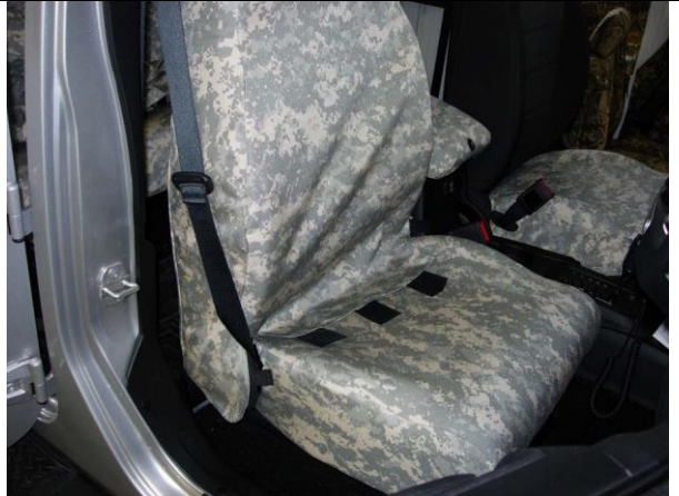
Step 16. Driver & Passenger Tops/DT&PT: Slide the cover on with the extending hook Velcro™ to the front.
