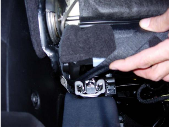
Step 13. Driver & Passenger Bottoms/DB&PB: Route the far back side Velcro™ where shown, above the seat slide in back.
