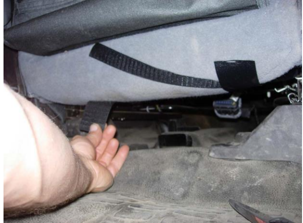
Step 18. Driver & Passenger Bottoms/DB&PB Mate the Velcro's to the carpet on the seat.
