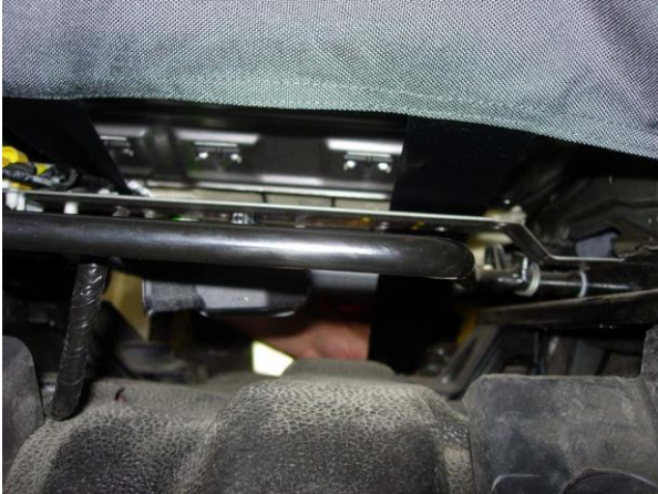
Step 17. Driver & Passenger Bottoms/DB&PB Route the long front Velcro's under the seat as shown, above the metal framework.
