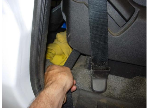
Step 14. Driver & Passenger Bottoms/DB&PB Feel for the Velcro under the plastic and slide it free.
