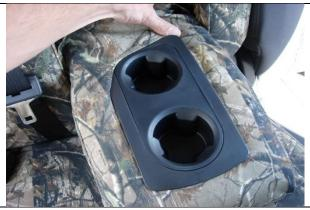
**Step 10.** Armrest/A: Slide the cover on with the cut-out on the top, and extending hook Velcro<sup>™</sup> to the front. Tuck it under the front of the drink holders, then the back.
