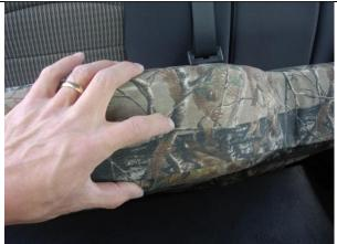
**Step 14. Driver & Passenger Bottoms/DB&PB:** Work the fabric from the seams inside the cover to the middle (pointer finger), and line up the seams.
