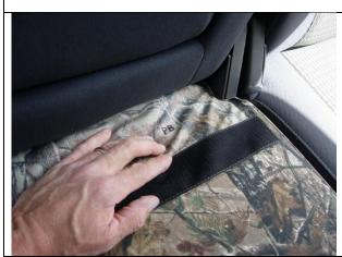
**Step 13. Driver & Passenger Bottoms/DB&PB:** Tilt the seat bottom up, and slide the seat covers on with the letters "DB" & "PB" up.
