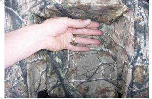
**Step 9. Driver & Passenger Top/DT&PT:** Push the fabric into the top of the cavity with one hand, and then mate the loop Velcro<sup>™</sup> in back by pressing it down onto the hook Velcro<sup>™</sup> behind the armrest with the other hand.
