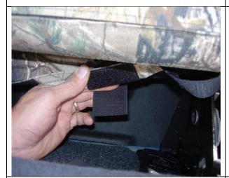
Step 7. Passenger Top/PT: Reach up behind the seat and feel for the long hook Velcro<sup>™</sup> from Step 3, and pull them down. Slide your hand down the front of the seat gathering up slack. Pull the seat cover all the way to the back edge of the seat (under the seat), connecting the hook Velcro<sup>™</sup> to the loop (fuzzy) Velcro<sup>™</sup> sewn inside the front edge.
