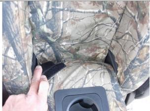
Step 11. Armrest/A: Pull the hook Velcro<sup>™</sup> up from the back and mate them to the loop Velcro<sup>™</sup> sewn inside the back edge.
