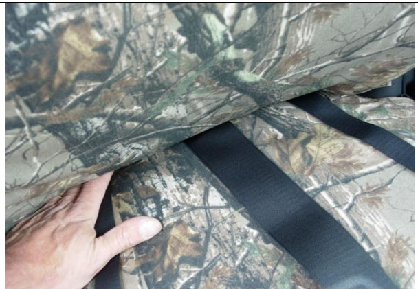
Step 12. Driver & Passenger Top/DT&PT: Tuck the hook Velcro™ into the seat, slide the seat forward and tip the backrests forward.
