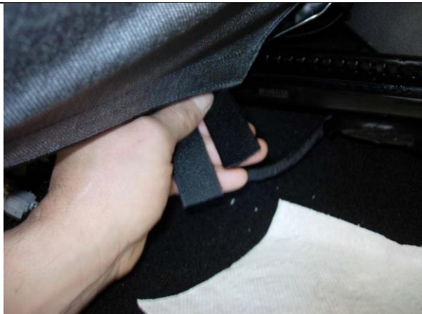
Step 15. Driver & Passenger Top/DT&PT: Re-connect the plastic clips under the seat. Route the 1"x12" loop Velcro™ over the same metal bar used in Step 13 and pull both ends out to the back.
