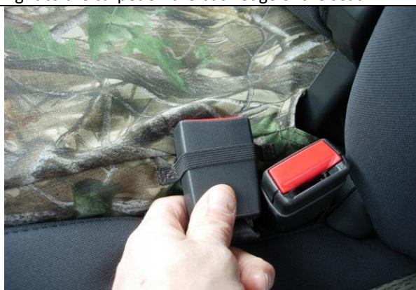
Step 20. Middle Bottom/MB: Push the seat belts through the provided elastic loops on the seat cover.
