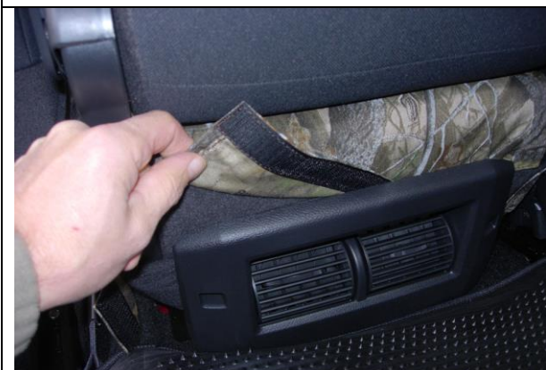
Step 19. Middle Bottom/MB: Pull the cover back and press the hook Velcro™ to the carpet on the back edge of the seat.
