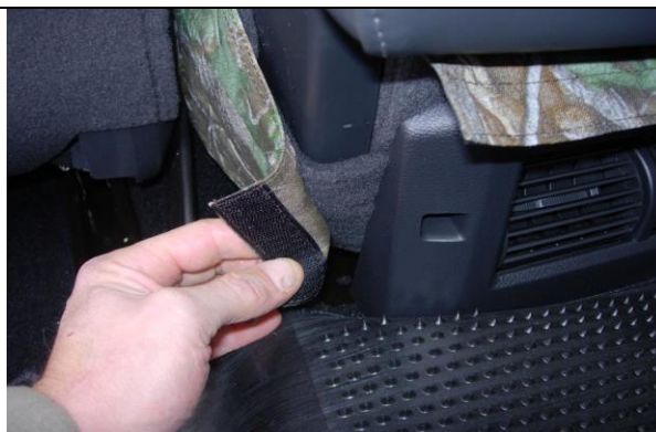
Step 18. Middle Bottom/MB: Line up the seams of the seat cover to the seams of the seat, and then press the hook Velcro™ on left and right to the carpet on the back edge of the seat.
