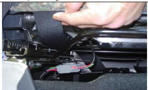
**Step 4. Driver & Passenger Bottoms/DB&PB:** All the parts of the seat cover are labeled inside. Use the Seat Cover Piece Identification Chart to ID parts. Tuck the back edge of the seat cover into the seat. Next, route the long hook (sticky) fasteners under the front of the seat where shown, avoiding any seat mechanisms.
