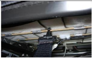
**Step 9. Driver & Passenger Bottoms/DB&PB:** Connect the plastic hooks under the back edge of the seat to the metal bar, and then mate hook fasteners to the loop fastener as in Step 7. This will keep the seat cover from shifting around. Trim off the excess length of fasteners.
