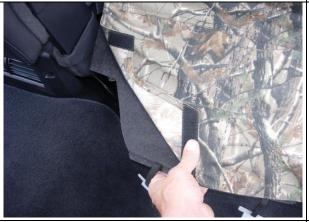
**Step 15. Driver & Passenger Top/DT&PT:** Center the backside of the seat cover and mate the hook fasteners on the seat cover to the carpet on the back of the seat. Lastly, re-connect the plastic clips under the seat.
