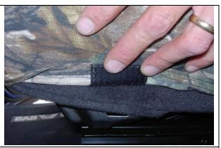
Step 7. Driver & Passenger Bottoms/DB&PB: Mate the long front edge hook fasteners to the loop fastener sewn on the back edge. Route the outside edge hook fastener at an angle and mate it to the loop fastener sewn on the back edge. Use one hand in a smoothing action from front to back along the outside edge and top of the seat cover while pulling on the back of the seat cover, then tightening the fasteners.
