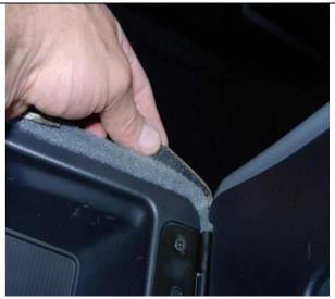
**Step 22. Console/C:** Pull the back left & right sides up and press the Velcro<sup>™</sup> to the carpet as shown.
