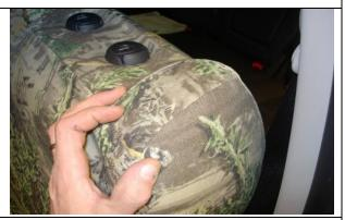
**Step 10. Driver & Passenger Top/DT&PT:** Slide the seat covers on with the extending hook fasteners to the front. Tuck the fabric under the plastic on the outside edge of the seat. Like Step 6, line up the seams of the seat cover to the seams of the seat.
