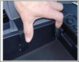
Step 23. Console/C: Slide the rear Velcro<sup>™</sup> into the hinge area using a sawing motion while moving the lid. Fold the Velcro<sup>™</sup> into the cavity and look where they will lay inside. Clean the areas with rubbing alcohol by scrubbing hard and wiping it dry while it's still wet. Pull the Velcro<sup>™</sup> tight, peel off the backing and press the adhesive Velcro<sup>™</sup> onto the plastic.
