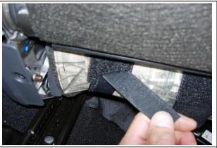
**Step 14. Driver & Passenger Top/DT&PT:** Use one hand in a smoothing action down the front of the seat, pull the fabric down in back and hold it to the seat while you pull the Velcro<sup>™</sup> forward over the bar, then bring it back and connect the Velcro<sup>™</sup> as shown. It might take a couple tries before you get it tight.
