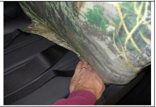
**Step 12. Driver & Passenger Top/DT&PT:** Tuck the hook fasteners into the seat, slide the seat forward and tip the backrests forward.
