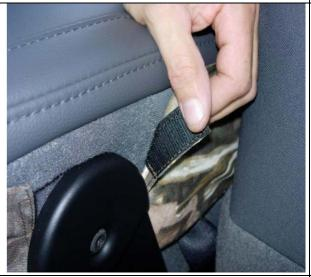
**Step 21. Console/C:** Pull the back left & right sides up and press the Velcro<sup>™</sup> to the carpet as shown.
