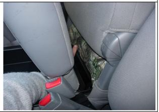
**Step 16. Middle Bottom Back/MBB:** Lift the middle bottom up and place the loop Velcro<sup>™</sup> into the cavity of the middle bottom. Prepare the surface of the plastic with rubbing alcohol. Press the adhesive hook Velcro<sup>™</sup> to the inside of the plastic box.
