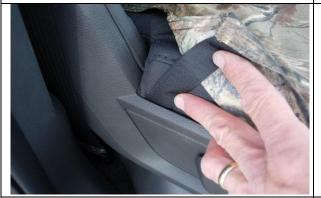
**Step 5. Driver & Passenger Bottoms/DB&PB:** Slide the long outside edge hook fasteners in as shown between the plastic and the seat, then put the seat belts through the elastic on the inside of the cover.
