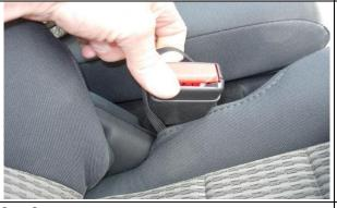
**Step 3.** Remove the seat belt from the elastic on the inside edge of the driver and passenger seat bottoms.
