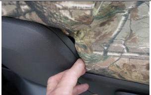
**Step 6. Driver & Passenger Bottoms/DB&PB:** Line up the seams of the seat cover to the seams of the seat, they should match closely. Then, tuck the outside edge in as shown.
