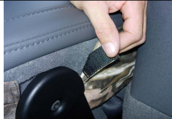
Step 21. Console/C: Pull the right side up and press the Velcro™ to the carpet.
