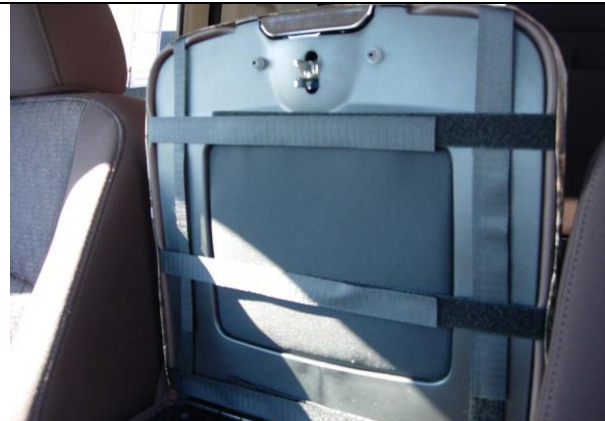
Step 26. Lid/L: Carefully open the Velcro™ and fold the console down, place the cover on and open the lid. Line up the seams and connect the Velcro™ under the lid as shown.
