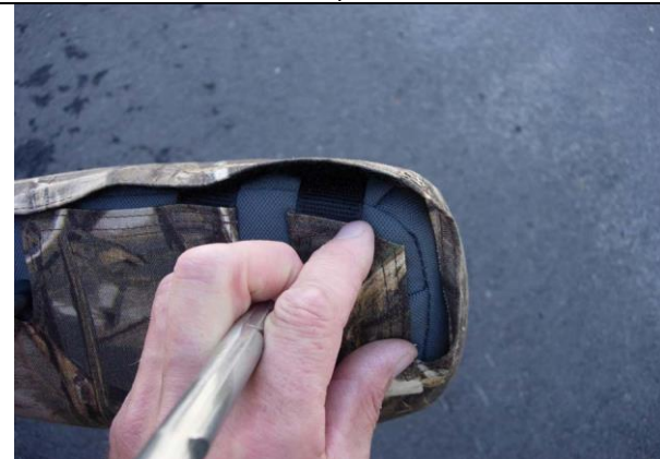
Step 25. Headrests/H: Tuck the front Velcro™ under the back edge and connect it to the loop Velcro™ sewn inside the back edge.
