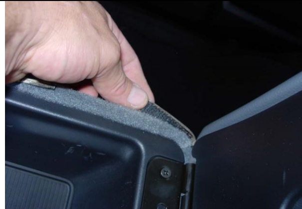
Step 22. Console/C: Pull the back left & right sides up and press the Velcro™ to the carpet as shown.
