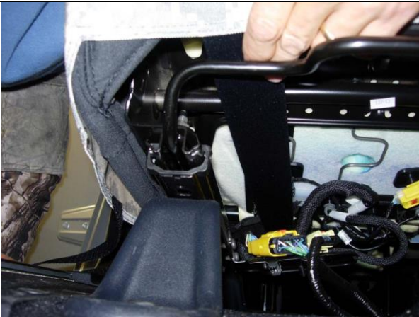
Step 9. Driver & Passenger Bottoms/DB&PB: Route the under the knee Velcro™ above the wiring.
