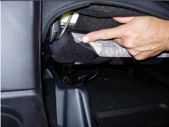
Step 15. Driver & Passenger Bottoms/DB&PB: Pull the back edge of the cover back hard and connect it to the carpet on the back edge of the seat. Skip this step if no carpet exists on the seat. If no carpet exists, snap the two buckles under the seat and press them to the loop Velcro™ sewn on the back edge.
