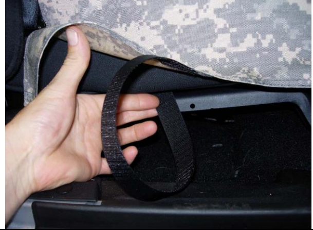
Step 12. Driver & Passenger Bottoms/DB&PB: Route the side hook Velcro™ over the seat slides.
