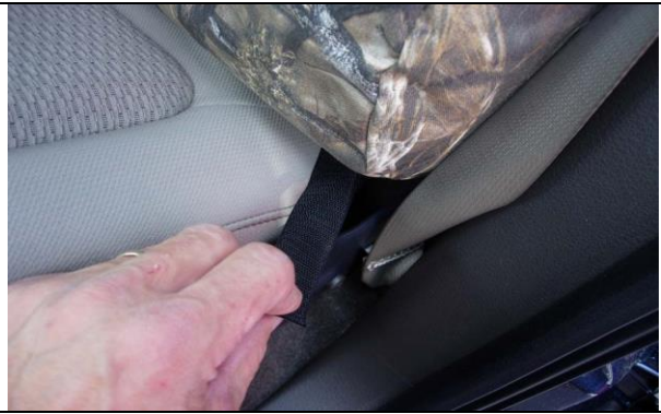
Step 8. Top/T: Tuck the long front right and left hook Velcro™ into the seat, around the inside of the outside child restraint.
