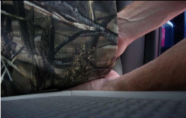
Step 9. Top/T: Using two hands, route the long left and right hook Velcro™ and press them to the loop Velcro™ sewn on the side of the seat covers.
