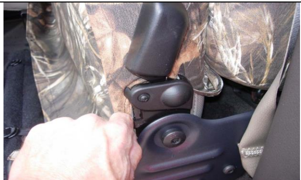
Step 12. Driver & Passenger Bottom/DB& PB: Tuck the cover behind the plastic on the sides.
