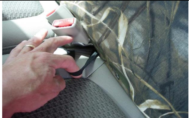
Step 10. Driver Bottom/DB: Remove the two female seat belt ends from the factory restraint.
