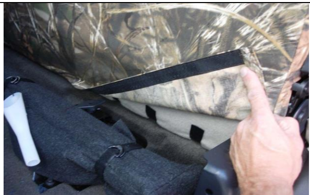
Step 14. Driver & Passenger Bottom/DB& PB: Lastly, press the bottom side Velcro™ as shown.
