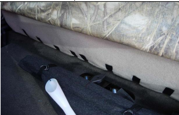
Step 13. Driver & Passenger Bottom/DB& PB: press the top side Velcro's first as shown.
