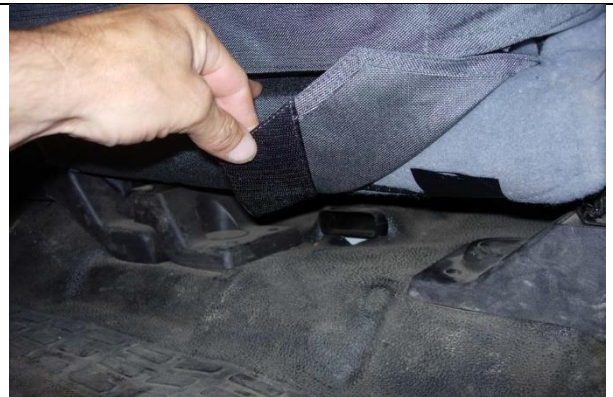
Step 18. Driver & Passenger Bottoms/DB&PB Pull the rear part of the seat cover back while using one hand in a smoothing action from front to back and press it to the carpet on the seat.
