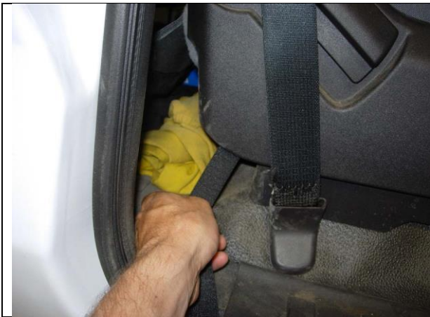
Step 13. Driver & Passenger Bottoms/DB&PB Feel for the Velcro™ under the plastic and slide it free.
