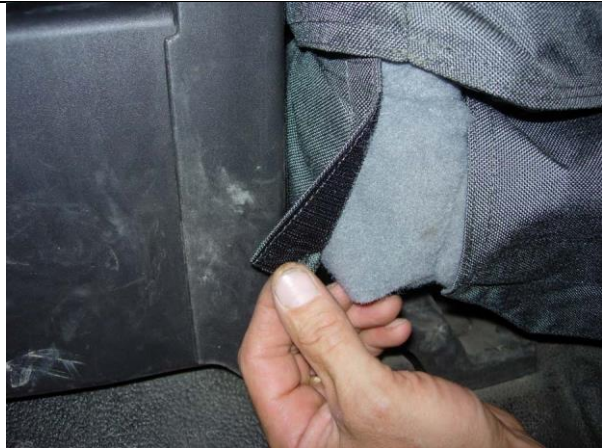
Step 15. Driver & Passenger Bottoms/DB&PB Pull the inside edge next to the console around to the back and press it to the carpet on the seat. You may have to release the side Velcro™ from the carpet in order to get it back. Next, route the long side Velcro™ in front of the seatbelt next to the console by folding it in half lengthwise and poking it thru. Do not put your fingers under the seat while poking it thru, this is the sharpest area under the seat. Look for it behind the seat and carefully grab it, connect same as Step 14.
