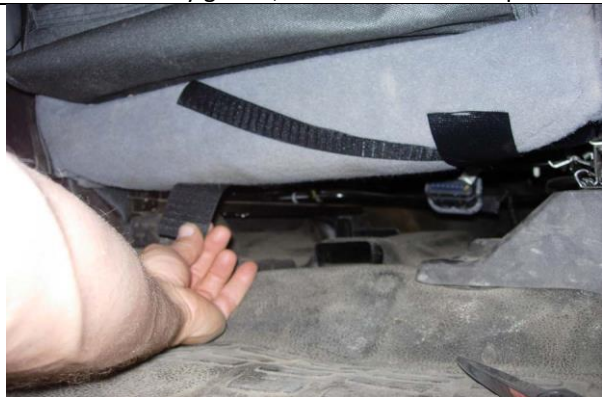
Step 17. Driver & Passenger Bottoms/DB&PB Pull back and press the Velcro™ to the carpet on the back edge of the seat.
