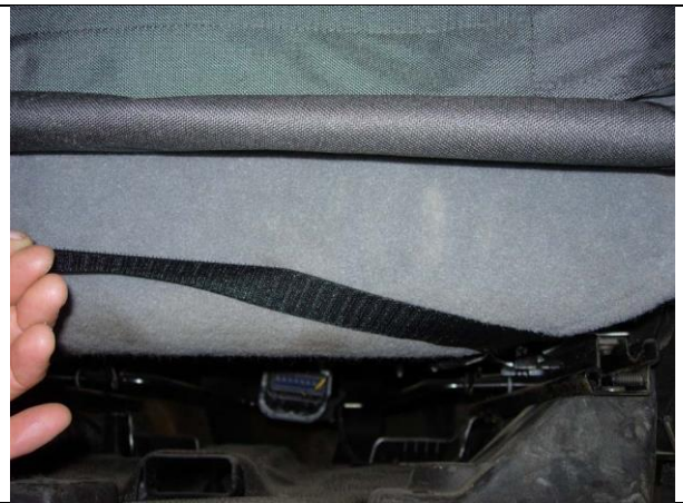
Step 14. Driver & Passenger Bottoms/DB&PB Route the Velcro™ around the back corner of the seat and press it to the carpet on the back edge of the seat.
