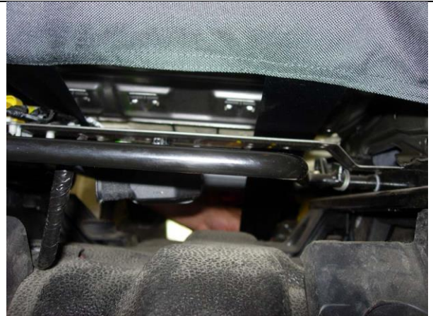
Step 16. Driver & Passenger Bottoms/DB&PB Route the long front Velcro™ under the seat as shown, above the metal framework. Do this by folding them in half lengthwise with the sticky facing in. It'll stiffen them up so your able to poke them thru all the way to the back.
