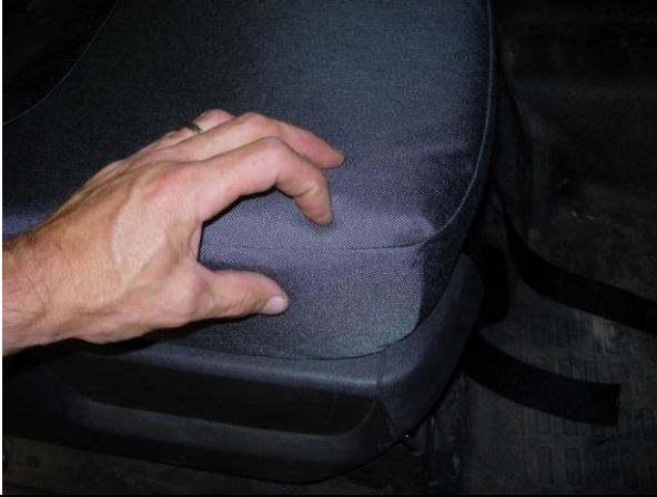
Step 11. Driver & Passenger Bottoms/DB&PB Work the fabric inside the seat cover from forefinger to thumb, or outward, line up the seams like Step 3.
