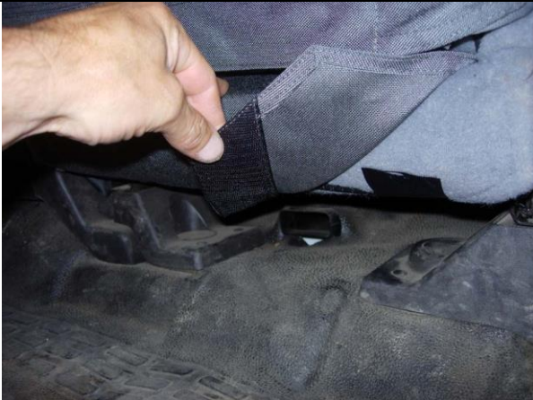
Step 19. Driver & Passenger Bottoms/DB&PB Pull the rear part of the seat cover back while using one hand in a smoothing action from front to back
