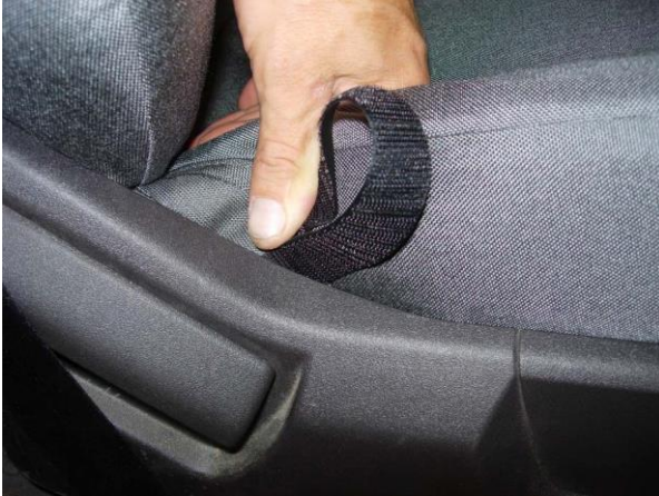
Step 13. Driver & Passenger Bottoms/DB&PB Tuck the long outside edge Velcro in where shown. folding the Velcro™ in half lengthwise helps it not stick to the seat, reduces size to 1/2", and makes it stiffer.
