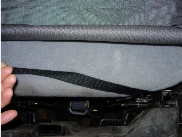
Step 15. Driver & Passenger Bottoms/DB&PB Route the Velcro around the back corner of the seat and mate it to the carpet on the back edge of the seat.
