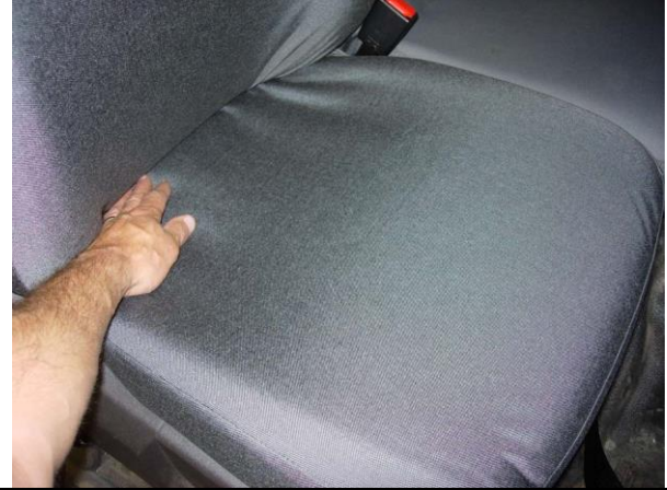
Step 12. Driver & Passenger Bottoms/DB&PB Tuck in the back edge of the seat cover.
