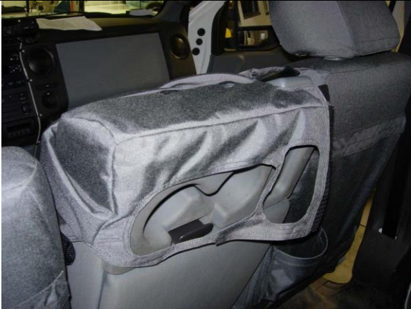
Step 21. Console/C With the console up, slide the cover on with the cut-outs on top.
