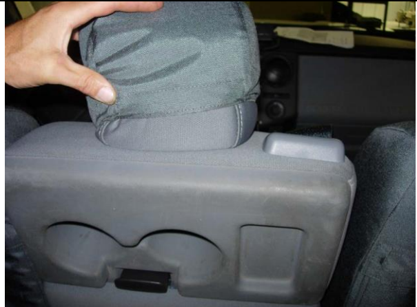
Step 20. Console/C Slide the headrest cover on with the extending Velcro to the front while it's on the console. Mate the fasteners as in Step 3. Remove headrest as in Step 2.
