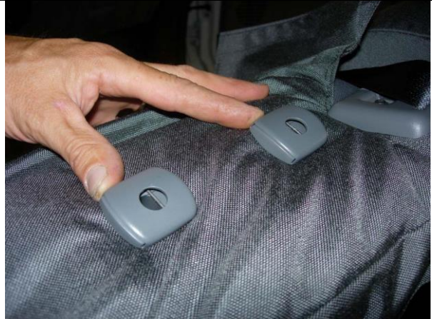
Step 22. Console/C Tuck the fabric under the plastic of the headrests, and the shoulder seat belt.
