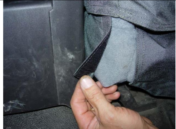
Step 16. Driver & Passenger Bottoms/DB&PB Pull the inside edge next to the console around to the back and mate it to the carpet on the seat. You may have to release the side Velcro's from the carpet in order to get it back.
