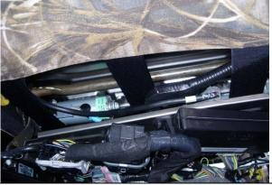
**Step 14. Driver & Passenger Bottom/DB&PB:** Route the long hook Velcro<sup>™</sup> under the front of the seat, over the top of the metal framework to the back edge of the seat.
