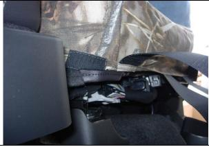
**Step 6. Driver & Passenger Bottom/DB&PB:** Turn the inside edge of the seat cover next to the console inside out to help keep the Velcro™ from sticking while you work the rest of the seat cover.
