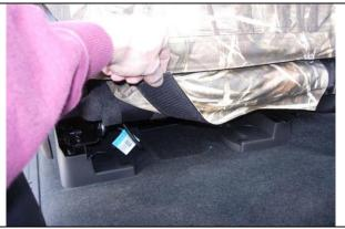
Step 16. Driver & Passenger Bottom/DB&PB: Again, use one hand in a smoothing action from front to back while pulling on the rear part of the seat cover. Connect it to the carpet on the back edge of the seat, starting on one side, moving to the other.
