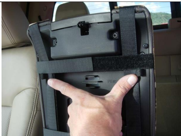
Step 22. Lid/L Lastly, connect the side to side Velcro™, making sure to keep the front Velcro™ inside of the plastic studs.
