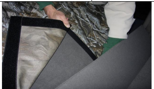
Step 14. Passenger Top/PT: Continue connecting the Velcro™ using slight downward pressure, all the way to the bottom.
