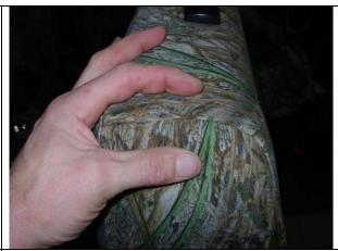
**Step 8. Driver & Passenger Top/DT&PT:** Manipulate the material inside the seat cover from thumb to forefinger on top and down both front sides. As in Step 2, align the seams of the seat cover left and right to the seams of the seat, they should closely match.
