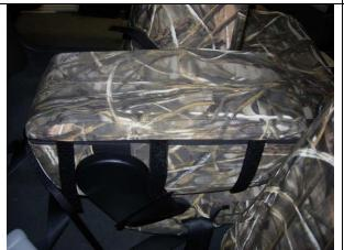
**Step 17. Lid/L:** With the console down, open all the Velcro<sup>™</sup> and place the lid cover on with the letter "L" to the back.
