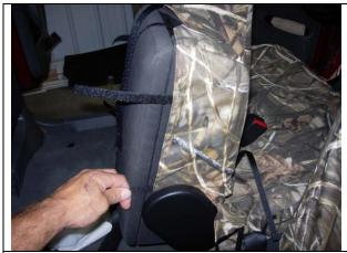
**Step 13. Console/C:** With the console up, slide the cover on and tuck the fabric in around the hinge area.
