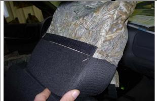
**Step 1. Headrests/H:** All the parts of the seat cover are labeled on the inside right corners of the seat cover. Use the seat cover part ID chart to identify part numbers. Turn the hook Velcro<sup>™</sup> inside out on the back of the headrest covers and slide it down into position.
