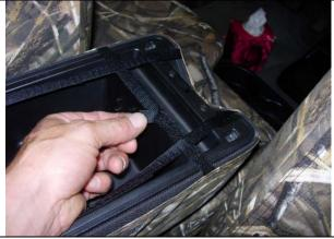
**Step 15. Console/C:** Tightly connect these two side to side Velcro<sup>™</sup> in front.
