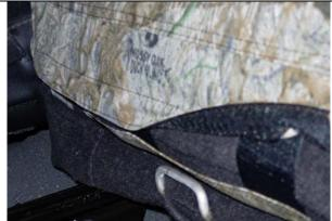
**Step 12. Driver & Passenger Top/DT&PT:** Pull down and press the back edge Velcro<sup>™</sup> onto the carpet on the seat back starting in the middle and work your way out.
