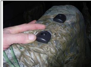
**Step 7. Driver & Passenger Top/DT&PT:** Tuck the fabric of the seat cover under the plastic for the headrests, starting with the push button side first.
