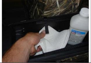
**Step 16. Console/C:** Dry fit the remaining Velcro<sup>™</sup> by laying them into the box. Clean those areas with rubbing alcohol by scrubbing hard then wiping dry while it's still wet.
