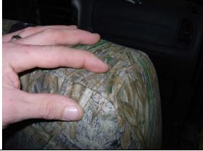
**Step 9. Driver & Passenger Top/DT&PT:** Manipulate the fabric inside the seat cover from thumb to forefinger around the backside corners.
