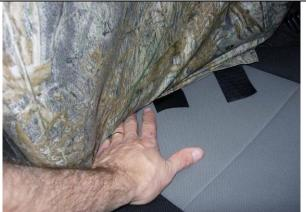
**Step 10. Driver & Passenger Top/DT&PT:** Tuck the front edge hook Velcro<sup>™</sup> into the seat and fold the seat forward.
