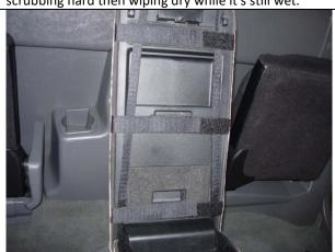
**Step 18. Lid/L:** Open the lid up and connect the Velcro<sup>™</sup> underneath starting with the front to back ones first (or top to bottom as seen in the picture), then the side to side Velcro<sup>™</sup>. Re-tighten Velcro<sup>™</sup> as needed for best fit.
