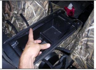
**Step 14. Console/C:** Slide the rear Velcro<sup>™</sup> in next to the hinge and connect them to the long front Velcro<sup>™</sup>. Re-tighten the Velcro<sup>™</sup> if needed to make sure they're really tight.
