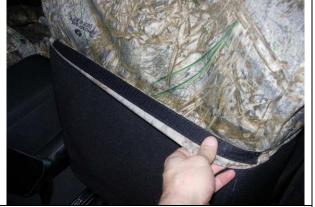
**Step 6. Driver & Passenger Top/DT&PT:** As done with the headrest cover, turn the backside hook Velcro<sup>™</sup> inside out while sliding the seat cover down over the backrest.
