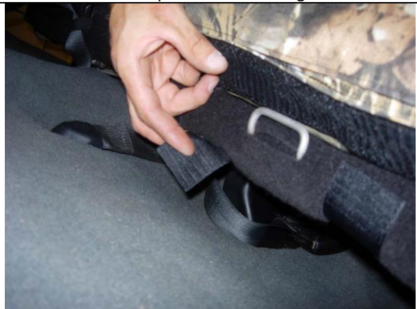
Step 18. Driver & Passenger Bottom/DB&PB: Route the hook Velcro™ under the seat and connect them to the carpet on the back of the seat.
