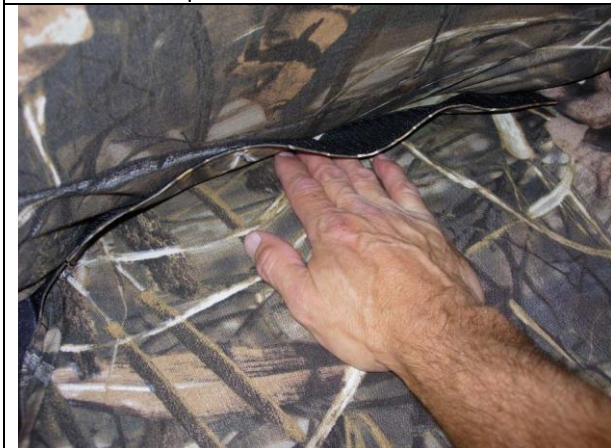
Step 17. Driver & Passenger Bottom/DB&PB: Tuck the back edge of the seat cover in.
