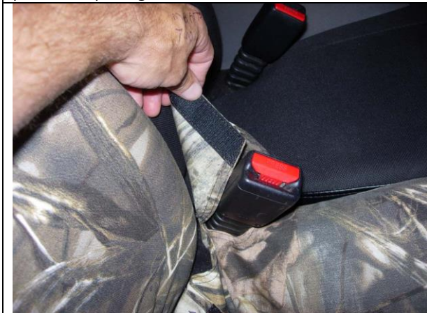
Step 15. Driver & Passenger Bottom/DB&PB: Tuck the inside piece of material thru to the back.
