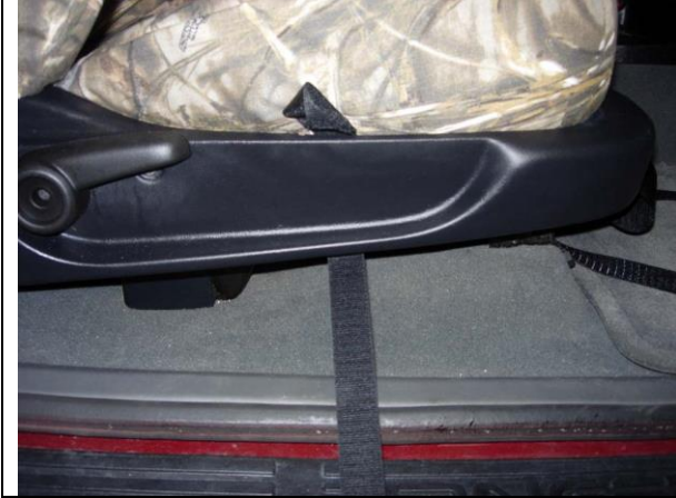
Step 19. Driver & Passenger Bottom/DB&PB Slide the long side Velcro™ behind the plastic cowling.
