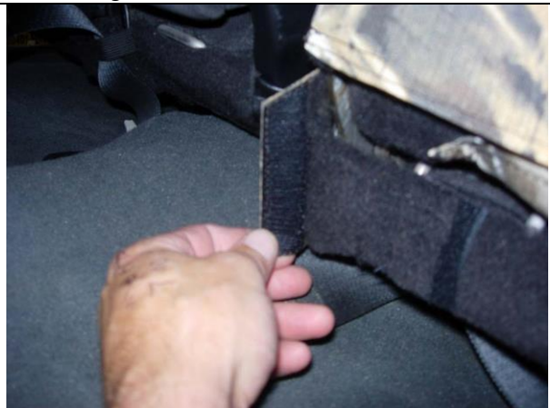
Step 16. Driver & Passenger Bottom/DB&PB: Connect it to the carpet on the back edge of the seat.
