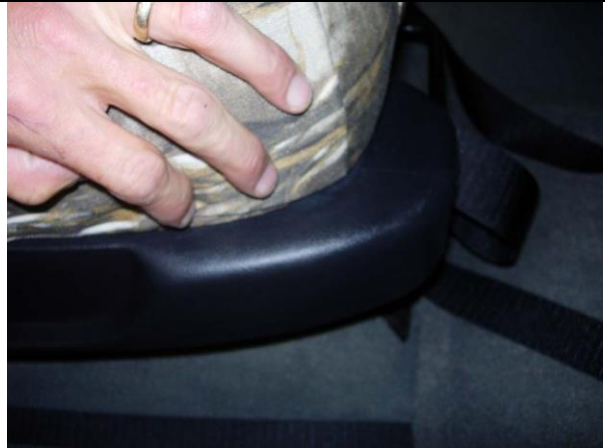
Step 14. Driver & Passenger Bottom/DB&PB: Tuck the fabric behind the plastic cowl along the outside edge.
