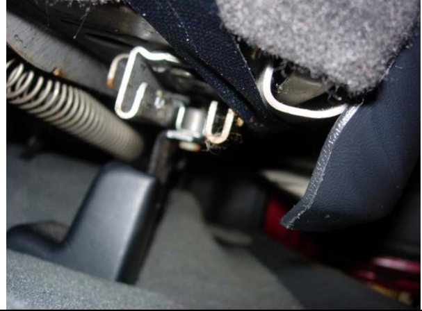
Step 20. Driver & Passenger Bottom/DB&PB: Route the side Velcro™ over top the seat slide, unlike the picture. The picture shows the top right of the slide being covered by the Velcro™. Tuck it over the slide, and connect it to the carpet on the back of the seat. Lastly, pull the rear edge of the seat back and press it to the carpet on the back edge of the seat.
