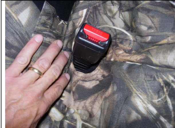
Step 13. Driver & Passenger Bottom/DB&PB: Place the seat cover on and poke the seat belt thru the provided opening.
