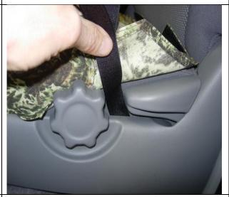
Step 4. Driver and Passenger Bottom/DB&PB: Slide 4-5" of the long outside edge hook Velcro™ where shown between the seat and the plastic.
