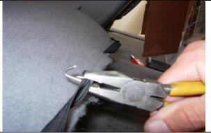
**Step 11. Driver and Passenger Top/DT&PT:**For 2005-08: Using pliers, clamp the provided metal hooks to the elastic straps with the hook up. Connect the hooks under the seat to the metal bar.
