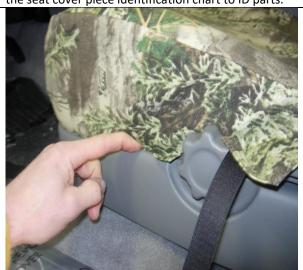
**Step 3. Driver and Passenger Bottom/DB&PB**: Tuck the fabric behind the plastic on the outside edge.
