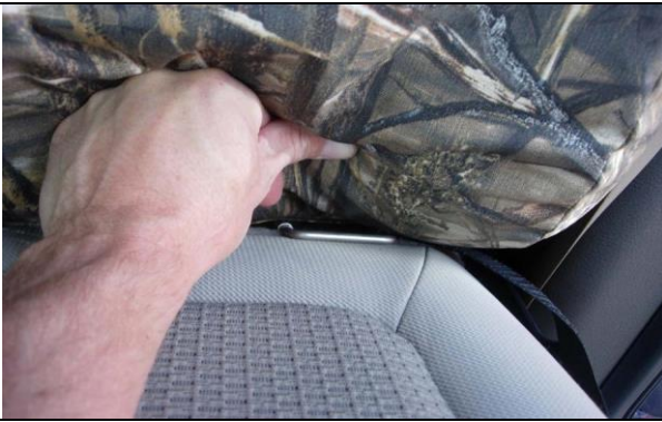
Step 7. Top/T: Tuck the seat cover between the seat and the four child restraints.
