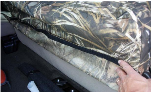
Step 11. Driver & Passenger Bottom/DB& PB: Slide the covers on with the seat cover turned up and the hook Velcro™ away from the seat bottom.
