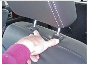
Step 1. Driver & Passenger Top/DT&PT: Temporarily remove the headrests by lifting them up all the way. Then, keeping gentle upward pressure, push the release buttons at the same time until the headrest comes out.
