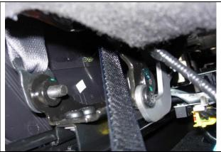
Step 11. Driver & Passenger Bottom/DB&PB: View from under the back of the driver seat. Carefully feel for the Velcro™ under the seat, routing it where shown at an angle to the back.
