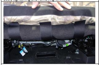
**Step 15. Driver & Passenger Bottom/DB&PB:**Mate them to the carpet on the back edge of the seat.
