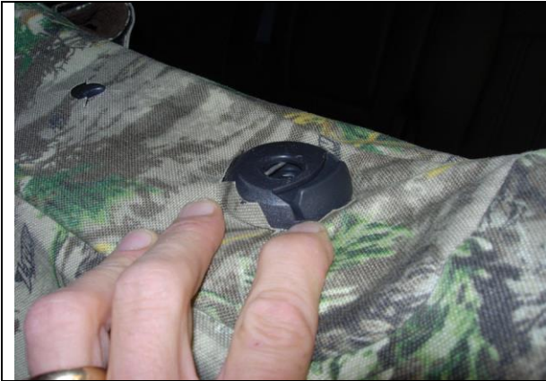
Step 11. Driver & Passenger Top/DT&PT: Tuck the fabric under the plastic of the headrests starting with the push button side as shown.
