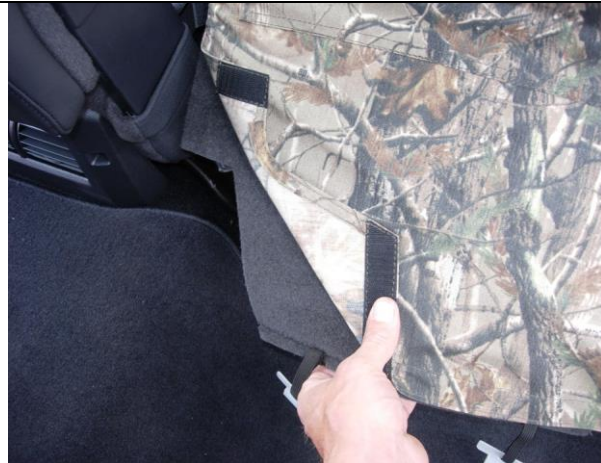
Step 15. Driver & Passenger Top/DT&PT: Center the backside of the seat cover and mate the hook fasteners on the seat cover to the carpet on the back of the seat. Lastly, re-connect the plastic clips under the seat.
