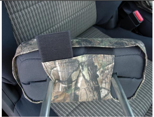
Step 23. Headrests/H: Slide the cover on with the extending hook fasteners to the front. Line up the seams, and mate the fasteners as shown.
