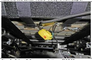
Step 9. Driver & Passenger Bottoms/DB&PB: Connect the plastic hooks under the back edge of the
