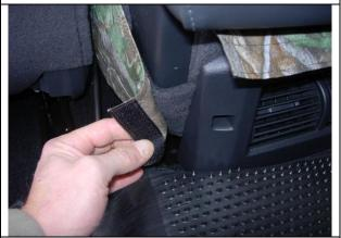
**Step 18. Middle Bottom/MB:** Line up the seams of the seat cover to the seams of the seat, and then press the hook Velcro<sup>™</sup> on left and right to the carpet on the back edge of the seat.
