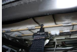
**Step 9. Driver & Passenger Bottoms/DB&PB:** Connect the plastic hooks under the back edge of the seat to the metal bar, and then mate hook Velcro<sup>™</sup> to the loop fastener sewn on the back edge. This will keep the seat cover from shifting around.
