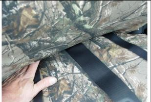
**Step 12.** Driver & Passenger Top/DT&PT: Tuck the hook Velcro<sup>™</sup> into the seat, slide the seat forward and tip the backrests forward.
