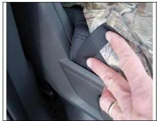
**Step 5. Driver & Passenger Bottoms/DB&PB:** Slide the long outside edge hook Velcro<sup>™</sup> in as shown between the plastic and the seat, then put the seat belts through the elastic on the inside of the seat cover.
