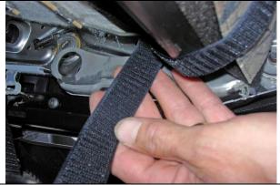
**Step 13. Driver & Passenger Top/DT&PT:** View from under the back of the seats. Route the long hook Velcro<sup>™</sup> on left and right, over the metal bar as shown. Do the same for the two inch wide center hook Velcro<sup>™</sup>.
