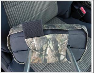
**Step 24. Headrests/H:** Slide the cover on with the extending hook Velcro<sup>™</sup> to the front. Line up the seams, and connect the Velcro<sup>™</sup> as shown.
