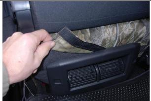
**Step 19. Middle Bottom/MB:** Pull the cover back and press the hook Velcro<sup>™</sup> to the carpet on the back edge of the seat.
