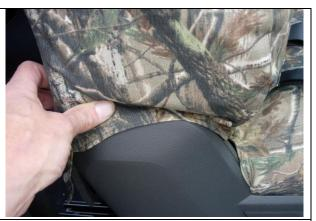
**Step 10. Driver & Passenger Top/DT&PT:** Slide the seat covers on with the extending hook Velcro<sup>™</sup> to the front. Tuck the fabric under the plastic on the outside edge of the seat. Like Step 6, line up the seams of the seat cover to the seams of the seat.
