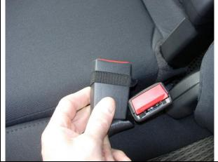
**Step 16. Middle Bottom/MB:** Remove the seat belt from the elastic on both sides of the middle bottom.
