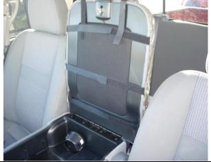
**Step 23. Lid/L:** Mate the Velcro<sup>™</sup> under the console lid starting with the top or front. The photo doesn't show the improvement to the top to bottom Velcro<sup>™</sup>. Slide the bottom, or rear Velcro<sup>™</sup> into the left and right side of the hinge, connecting them to the corresponding Velcro<sup>™</sup> in front.
