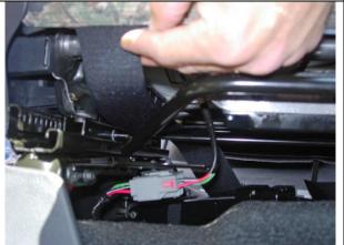
**Step 4. Driver & Passenger Bottoms/DB&PB:** All the parts of the seat cover are labeled inside. Use the Seat Cover Piece Identification Chart to ID parts. Tuck the back edge of the seat cover into the seat. Next, route the long hook (sticky) Velcro under the front of the seat where shown, avoiding any seat mechanisms.
