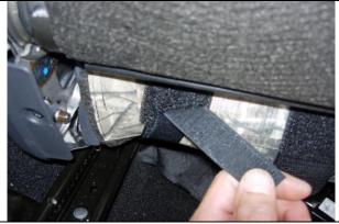
**Step 14. Driver & Passenger Top/DT&PT:** While gently pulling on the Velcro<sup>™</sup> from behind the seat, use one hand in a smoothing action down the front of the seat, and then press the hook Velcro<sup>™</sup> to the loop Velcro<sup>™</sup> sewn inside the seat cover.
