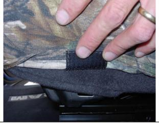
**Step 8. Driver & Passenger Bottoms/DB&PB:** View from the inside edge of the passenger bottom next to the middle bottom. Press the two hook Velcro<sup>™</sup> sewn inside the seat cover to the carpet on the seat. Like step 7, slide one hand from front to back along the inside edge while pressing the Velcro<sup>™</sup> to the carpet to remove any slack in the seat cover.
