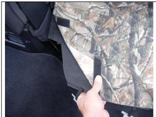
**Step 15. Driver & Passenger Top/DT&PT:** Re-connect the plastic clips under the seat. Center the backside of the seat cover and press the hook Velcro<sup>™</sup> onto the carpet on the back of the seat.
