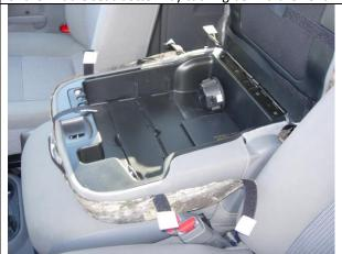
With the console in the up position, slide the console cover on and tuck it in on the bottom. Fold the console down, holding it in position with one hand. Note where the Velcro™ will lay inside the cavity. Fasten the right side and left side rear hook Velcro™ to the carpet behind the console hinge.
