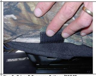
Step 8. Driver & Passenger Bottoms/DB&PB: View from the inside edge of the passenger bottom. Press the two hook Velcro™ sewn inside the seat cover to the carpet on the seat. Like step 7, slide one hand from front to back along the inside edge while connecting the Velcro™ to the carpet to remove any slack in the seat cover.
