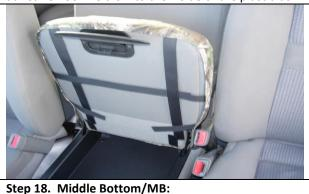
Connect the Velcro<sup>™</sup> to the carpet on the bottom of the seat and then the middle Velcro<sup>™</sup> to each other.
