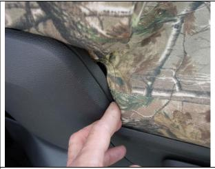
**Step 6. Driver & Passenger Bottoms/DB&PB:** Line up the seams of the seat cover to the seams of the seat, they should match closely. Then, tuck the outside edge in as shown.
