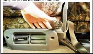
**Step 17. Middle Bottom Back/MBB:**Press the hook Velcro™ to the carpet on the back edge of the middle seat bottom by tucking behind the vent.
