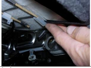
**Step 2.** (View from under the back of the seat bottom.) Temporarily unhook both plastic pieces sewn to the elastic straps by pushing them forward. Use caution reaching under the seat and avoid sharp metal edges.
