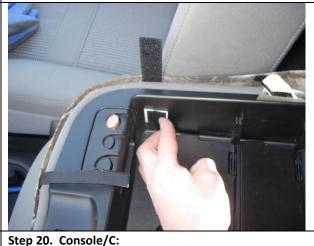
Clean the surface with rubbing alcohol as in Step 17.
