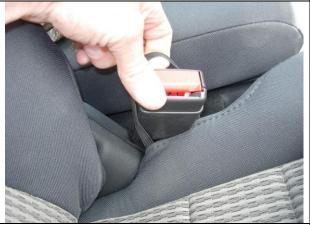
Remove the seat belt from the elastic on the inside edge of the driver and passenger seat bottoms.
