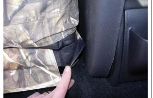
**Step 9. Driver & Passenger Bottom/DB&PB:** Pull the inside edge back, connecting the hook Velcro<sup>™</sup> to the carpet on the seat. Reach in next to the console and turn the seat cover right side out, connecting the Velcro<sup>™</sup> on the inside edge to the carpet on the seat.
