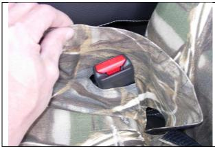
**Step 5. Driver & Passenger Bottom/DB&PB:** Place the seat cover on with the long hook Velcro<sup>™</sup> to the front. Put the seatbelt through the provided opening as shown.
