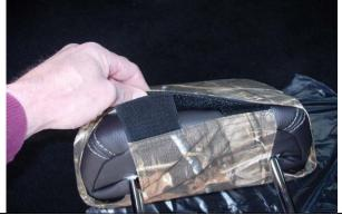
**Step 28. Headrest/H:** Tuck the hook Velcro<sup>™</sup> under the back edge, connecting the Velcro<sup>™</sup> as shown.
