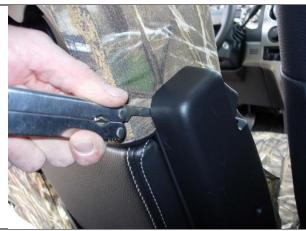
**Step 19. Console/C:** With the console in the up position, slide the cover on. With the cover pulled down all the way, carefully tuck the seat cover behind the plastic on the right side.
