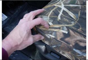
**Step 8.** Driver & Passenger Bottom/DB&PB: Then, work the material from the seam inside the seat cover outward (forefinger to thumb). Pulling the seat cover from behind the seat will help hold the cover to the front of the seat bottom.
