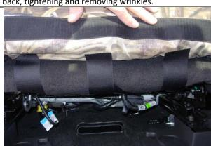
Step 15. Driver & Passenger Bottom/DB&PB: Connect them to the carpet on the back edge of the seat.
