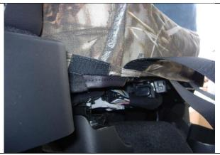
**Step 6.** Driver & Passenger Bottom/DB&PB: Turn the inside edge of the seat cover next to the console inside out to help keep the Velcro<sup>™</sup> from sticking while you work the rest of the seat cover.
