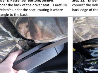
Step 13. Driver & Passenger Bottom/DB&PB: Tuck the outside edge of the seat cover in and back around the corner, connecting the hook Velcro<sup>™</sup> to the carpet on the seat similar to Step 9, while sliding one hand down the side of the seat cover from front to back, tightening and removing wrinkles.
