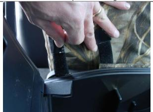
**Step 21. Console/C:** Use a sawing motion with the two Velcro<sup>™</sup> shown to help slide the seat cover behind the plastic on the left.
