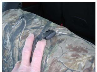
Step 3. Driver & Passenger Top/DT&PT: Slide the seat cover on with the extending hook (sticky) Velcro<sup>™</sup> to the front, and then tuck the fabric under the plastic of the headrests starting with the push button side first as shown. Line up the seams of the seat cover to the seams of your seats along the sides and top, they should closely match. connect the inside edge vertical Velcro<sup>™</sup> (not shown).
