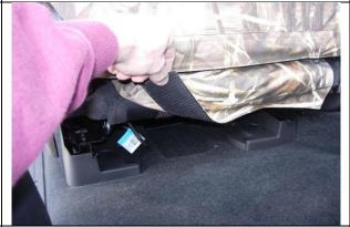
Step 16. Driver & Passenger Bottom/DB&PB: Again, use one hand in a smoothing action from front to back while pulling on the rear part of the seat cover. connect it to the carpet on the back edge of the seat, starting on one side, moving to the other.
