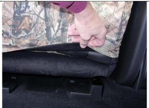
**Step 4. Driver & Passenger Top/DT&PT:** Tuck the hook Velcro<sup>™</sup> into the seat, gently pulling them through to the back. Use one hand in a smoothing action from top to bottom, down the front of the seat cover while gently pulling on the Velcro<sup>™</sup> from behind. Then tuck the hook Velcro<sup>™</sup> under the back edge, connecting them to the loop (fuzzy) Velcro<sup>™</sup> sewn inside the back edge.
