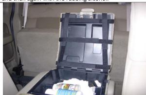
**Step 25. Lid/L:** Mate the Velcro<sup>™</sup> under the lid, re-connecting and tightening the fasteners for the best fit.
