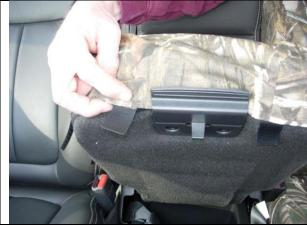
**Step 17. Middle Bottom/MB:** Place the cover over the front, tucking it behind the latch, connecting the Velcro<sup>™</sup> to the carpet in front.
