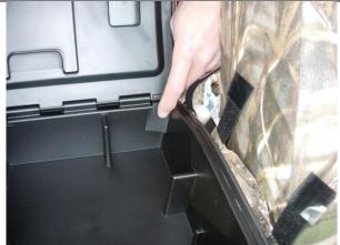
**Step 22. Console/C:** Again, use a sawing motion while moving the lid to slide the rear Velcro<sup>™</sup> into the hinge.
