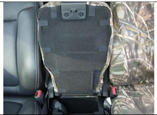
**Step 18. Middle Bottom/MB:** Again, use one hand in a smoothing action from front to back, and connecting the rear Velcro<sup>™</sup>. Slide one hand down the side, while connecting the Velcro<sup>™</sup>.
