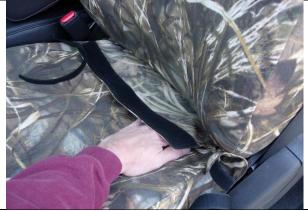
**Step 7.** Driver & Passenger Bottom/DB&PB: Tuck the back edge of the seat cover into the seat, but don't fasten it down yet. Line up the seams of the seat cover to the seams of your seats around the sides and front, they should closely match.
