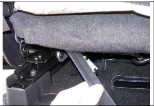
Step 12. Driver & Passenger Bottom/DB&PB: connect the Velcro<sup>™</sup> at an angle to the carpet on the back edge of the seat.
