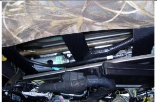
Step 14. Driver & Passenger Bottom/DB&PB: Route the long hook Velcro<sup>™</sup> under the front of the seat, over the top of the metal framework to the back edge of the seat.
