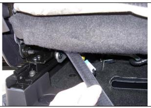
Step 12. Driver & Passenger Bottom/DB&PB: Mate the Velcro™ at an angle to the carpet on the back edge of the seat.
