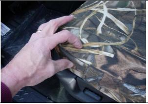
**Step 8. Driver & Passenger Bottom/DB&PB:**Then, work the material from the seam inside the seat cover outward (forefinger to thumb). Pulling the seat cover from behind the seat will help hold the cover to the front of the seat bottom.
