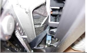
Step 8. Driver and Passenger Bottom/DB & PB: Route the outside edge hook Velcro™ between the metal frame and the seat mechanisms as shown and press it to the carpet on the back edge of the seat. Fasten the inside edge hook Velcro™ the same way.
