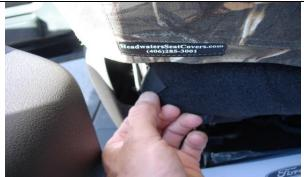
Step 9. Driver and Passenger Bottom/DB & PB: View from behind the driver's seat, bottom left. Tilt the backrest ahead and feed the short rear most outside edge hook Velcro™ around the back corner of the seat and press it to the carpet on the seat.
