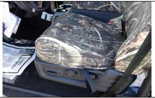
Step 5. Driver and Passenger Bottom/DB & PB: Place the seat covers on with the long 2" wide hook Velcro™ to the front. Pull the cover back into position and tuck in the back edge in but don't fasten it to the carpet yet. As in Step 2, line up the seams of the seat cover to the seams of the seat.
