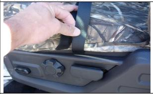
Step 7. Driver and Passenger Bottom/DB & PB: If the seats have electric controls, lift the seat all the way up towards the roof and forward. Slide the outside edge hook Velcro™ where shown between the seat and the plastic cowling.
