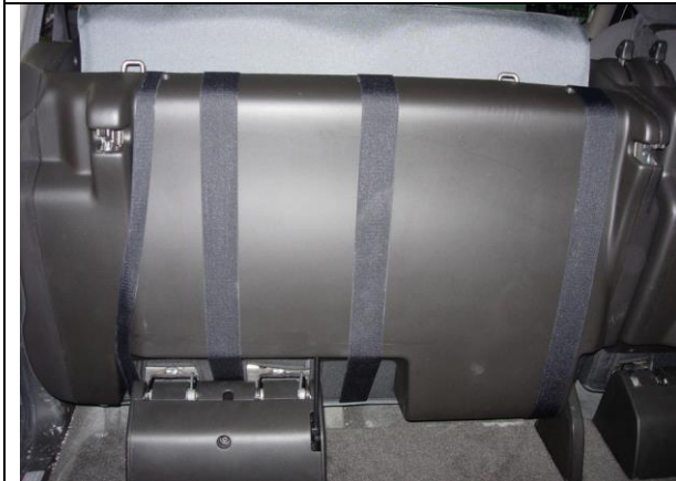
Step 7. Driver & passenger Bottoms/DB&PB: Connect them to the carpet on the back edge of the seat.
