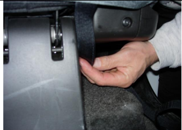
Step 6. Driver & passenger Bottoms/DB&PB: Route the front hook Velcro™ under the front of the seats.
