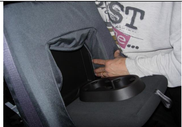
Step 10. Driver Top/DT: Line up the seams of the seat cover to the seams of the seat, they should closely match. Tuck the fabric behind the plastic on the left side.
