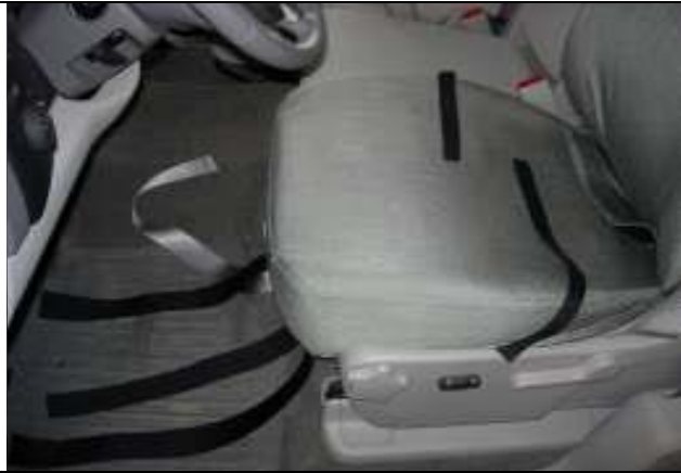
Step 7. Driver and Passenger Bottoms/DB&PB: Place the seat covers on with the long hook Velcro™ to the front.
