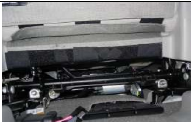
Step 11. Driver and Passenger Bottoms/DB&PB: If you have electric seats be sure to lift the seat up as high as it will go. This will pull everything away from your seat and free up some space. Route the three long hook Velcro™ in front under the seat and mate them to the loop Velcro™ sewn on the back edge. The moving metal parts under the seat have grease on them so check your hands for grease. Keep a rag handy for steps 11-15.
