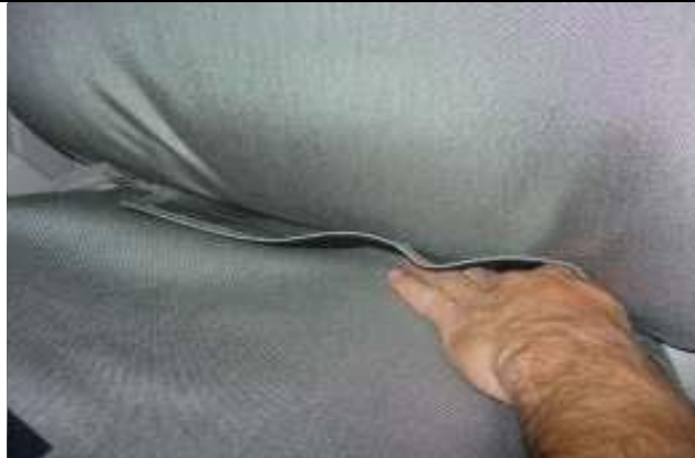
Step 9. Driver and Passenger Bottoms/DB&PB: Tuck the back edge of the seat cover into the seat. Pull it into position from behind the seat.
