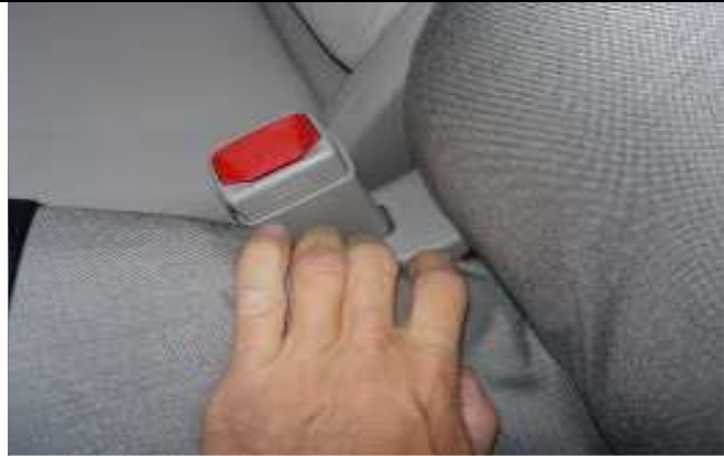
Step 10. Driver and Passenger Bottoms/DB&PB: Tuck the seat cover in behind the plastic on the inside back edge.
