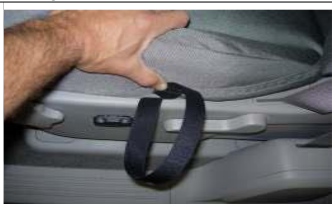
Step 12. Driver and Passenger Bottoms/DB&PB: Feed the long outside edge hook Velcro™ between the seat and the plastic. Feel for it under the seat, pull it tight and connect it at an angle to the loop Velcro™ on the back edge of the seat cover.
