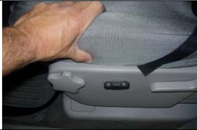
Step 8. Driver and Passenger Bottoms/DB&PB: Tuck the seat cover behind the plastic cowling.
