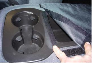
**Step 24. Lid/L:** Clean the surface of the plastic with rubbing alcohol. Peel off the backing and stick the adhesive hook to the plastic, pressing it hard into the plastic.
