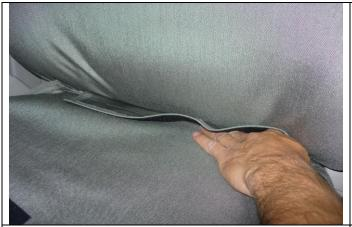
**Step 9. Driver and Passenger Bottoms/DB&PB:** Tuck the back edge of the seat cover into the seat. Pull it into position from behind the seat.
