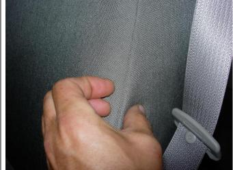
**Step 5. Driver and Passenger Tops/DT&PT**: Align the seams of the seat cover to the seams of the seat, they should match closely. Work the material from the seam inside the cover from the main body of the seat cover (fingers) to the middle (thumb). Do this for the front and back of the seat cover top.
