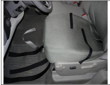
**Step 7. Driver and Passenger Bottoms/DB&PB:** Place the seat covers on with the long hook Velcro<sup>™</sup> to the front. As in Step 5 align the seams of the seat cover to the seams of the seat, they should match closely.
