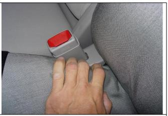
**Step 10. Driver and Passenger Bottoms/DB&PB:** Tuck the seat cover in behind the plastic on the inside back edge. Pull on the back edge of the seat cover.
