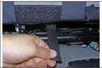
**Step 15. Driver and Passenger Bottoms/DB&PB:** Connect the plastic hooks under the back of the seat to the metal bar that supports the foam (about 2" in). Then, press the hook Velcro™ to the rear loop Velcro™. This will keep the seat cover from sliding forward, right, or left.
