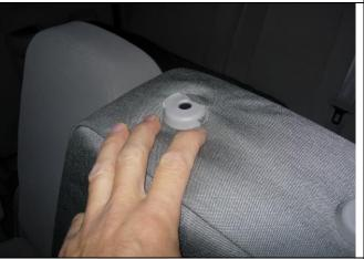
**Step 4. Driver and Passenger Tops/DT&PT:** Tuck the fabric of the seat cover under the plastic for the headrests starting with the push button side first as shown.
