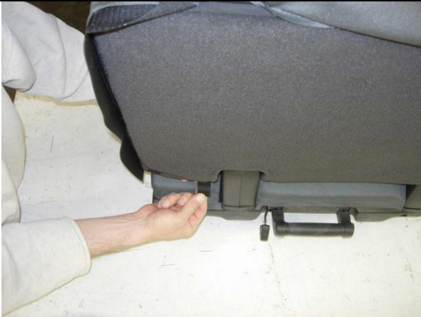
Step 15. Driver & Passenger Top/DT&PT: Pull the 1" hook Velcro™ through to the back and mate it to the carpet on the back of the seat.
