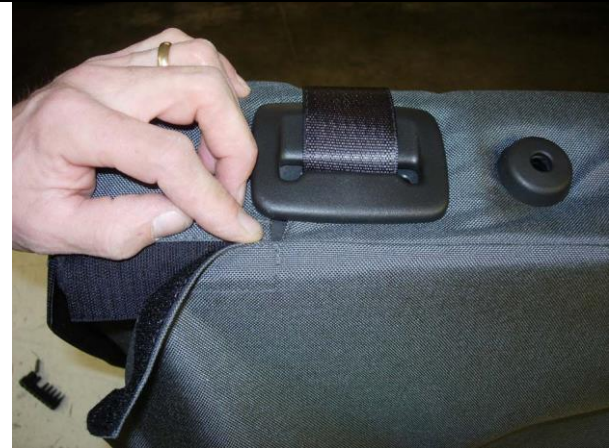
Step 14. Driver & Passenger Top/DT&PT: Tuck the seat cover under the plastic and mate the Velcro™.
