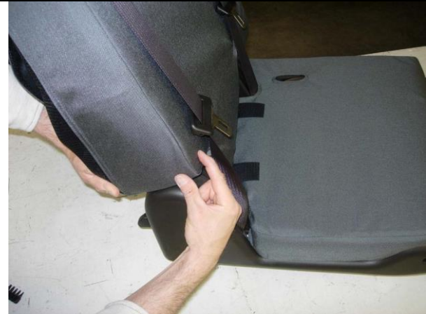
Step 16. Driver & Passenger Top/DT&PT: Form the sides of the seat cover to the seat by aligning the seams as in Step 5. Manipulate the material inside the seat cover from forefinger to thumb.
