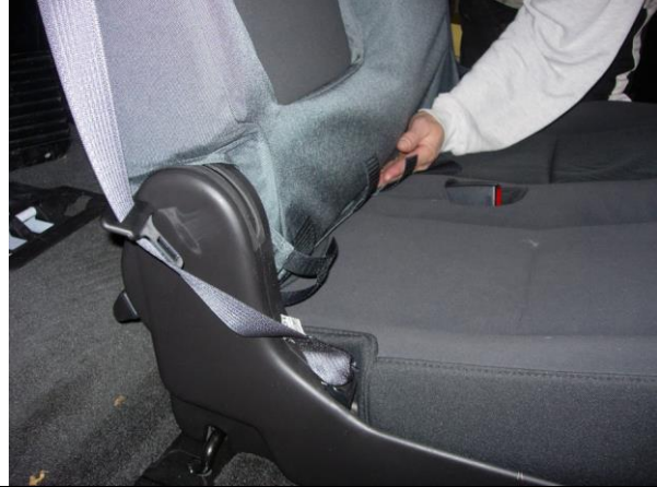
Step 13. Driver & Passenger Tops/DT&PT: Tuck the extending hook Velcro™ into the seat.
