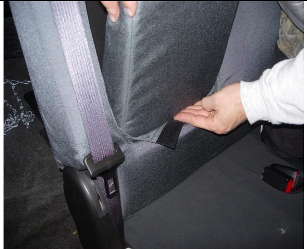
Step 22. Armrest-Console/A: Tuck the front edge in and fold the armrest down
