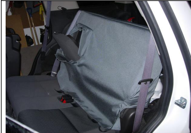
Step 9. Driver Top/DT: Very careful opening the inside edge of the seat cover. Place the cover on with the extending hook Velcro™ to the front. Fold the armrest out and tuck the seat cover around it.
