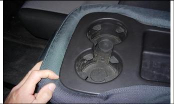
**Step 21. Armrest/A:** Slide the cover on with the large opening on top. Start by tucking the fabric under the plastic in front.
