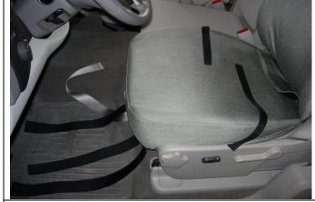
**Step 7. Driver and Passenger Bottoms/DB&PB:** Place the seat covers on with the long hook Velcro<sup>™</sup> to the front.
