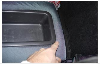
**Step 22. Armrest/A:** Tuck the fabric behind the plastic in back. This is a tight fit so you will have to pull hard and do one side at a time. Lastly, tuck the in the sides of the fabric.
