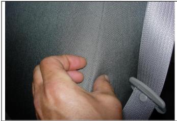
**Step 5. Driver and Passenger Tops/DT&PT**: Work the material from the seam inside the cover from the main body of the seat cover (fingers) to the middle (thumb). Do this for the front and back of the seat cover top.
