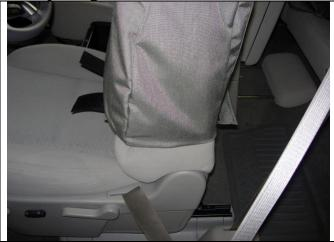
**Step 2. Driver and Passenger Tops/DT&PT:** Slide the seat covers on with the extending hook (sticky) Velcro<sup>™</sup> to the front. Notice how the seat compresses at its widest point. It will relax back out once it is pulled all the way down, and don't worry, you won't tear the seat cover apart pulling it down.
