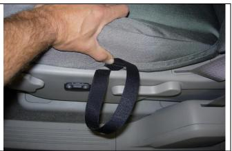
**Step 12. Driver and Passenger Bottoms/DB&PB:** Feed the long outside edge hook Velcro<sup>™</sup> between the seat and the plastic where shown. Carefully feel under the seat for the Velcro<sup>™</sup> in a gap between the seat slide and the seat frame. The seat slides have grease on them so clean your hands after doing this part.
