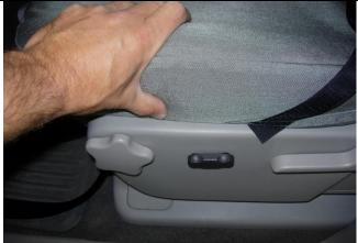
**Step 8. Driver and Passenger Bottoms/DB&PB:** Tuck the seat cover behind the plastic cowling on the outside edge.
