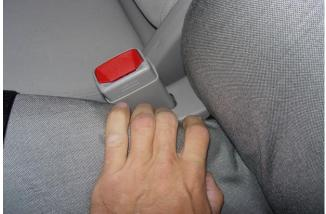
**Step 10. Driver and Passenger Bottoms/DB&PB:** Tuck the seat cover in behind the plastic on the inside back edge.
