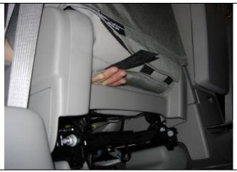
**Step 6. Driver and Passenger Tops/DT&PT:** Tuck the hook Velcro<sup>™</sup> into the seat and connect them to the loop (fuzzy) Velcro<sup>™</sup> sewn inside the back edge. Do it by sliding one hand down the front of the seat cover and push the hook Velcro<sup>™</sup> through as shown. Gently pull on the Velcro<sup>™</sup> from behind the seat with one hand and use the other hand in a smoothing action from top to bottom, then press then together.
