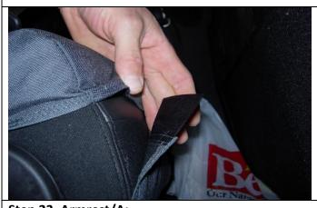
**Step 23. Armrest/A:** Tuck the hook Velcro<sup>™</sup> in and fold the armrest down, connecting the hook Velcro<sup>™</sup> to the loop Velcro<sup>™</sup> sewn inside the back edge.
