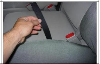
**Step 14. Driver and Passenger Bottoms/DB&PB:** Tuck the inside long hook Velcro<sup>™</sup> down in between the seats. Then, feel for it under the seat, pull it tight and connect it to the rear loop Velcro<sup>™</sup> at an angle.
