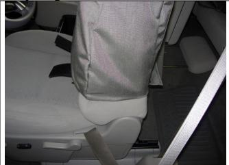
**Step 2. Driver and Passenger Tops/DT&PT:** Slide the seat covers on with the extending hook (sticky) Velcro<sup>™</sup> to the front. Notice how the seat compresses at its widest point. It will relax back out once it is pulled all the way down, and don't worry, you won't tear the seat cover apart pulling it down.
