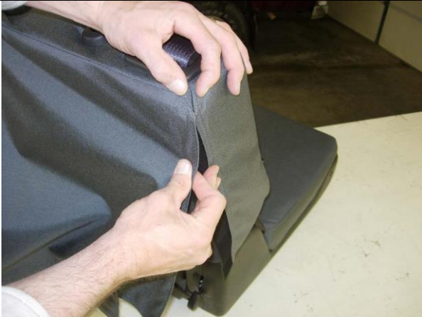
Step 17. Driver & Passenger Top/DT&PT: Mate the side Velcro™ starting at the top.
