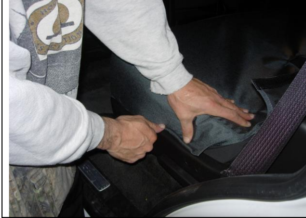
Step 5. Driver & passenger Bottoms/DB&PB: Tuck the outside edges of the seat cover behind the plastic cowl.
