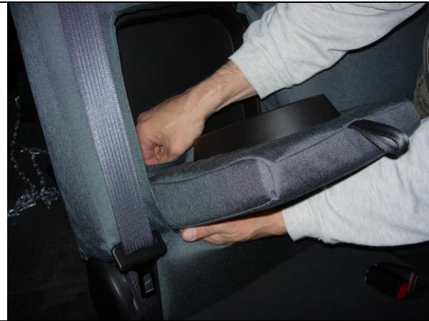
Step 23. Armrest-Console/A: Connect the Velcro™ at the back of the armrest.
