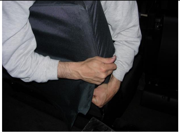
Step 16. Driver Top/DT: Continue working your way down using the "Bear Hug" method shown.
