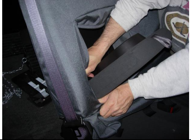
Step 12. Driver Top/DT: Tuck both side in and clear of the hinge area.
