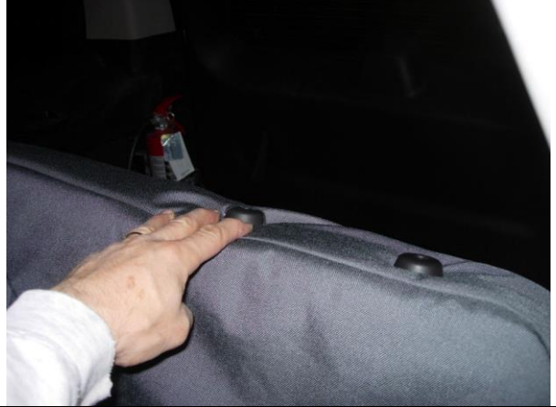
Step 14. Driver & Passenger Tops/DT&PT: Tuck the fabric under the plastic for the headrests.
