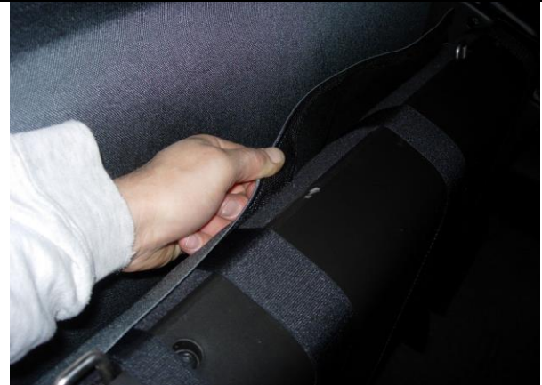
Step 8. Driver & passenger Bottoms/DB&PB: Pull the rear part of the seat cover back and connect it to the carpet on the back edge of the seat.
