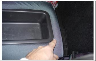
**Step 22. Armrest/A:** Tuck the fabric behind the plastic in back. This is a tight fit so you will have to pull hard and do one corner at a time. Lastly, tuck the sides in.
