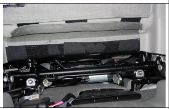
**Step 11. Driver and Passenger Bottoms/DB&PB:** If you have electric seats be sure to lift the seat up as high as it will go. This will pull everything away from your seat and free up some space. Route the three long hook Velcro<sup>™</sup> in front under the seat and connect them to the loop Velcro<sup>™</sup> sewn on the back edge. Avoid any seat mechanisms by keeping the Velcro<sup>™</sup> up and close to the seat bottom away from the metal framework.
