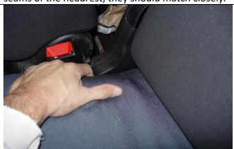
**Step 19. Middle Bottom/MB:** Smooth the side of the seat cover from front to back. Once in position, tuck the left and right rear sides in and mate the hook Velcro<sup>™</sup> sewn inside the cover to the carpet on the seat.
