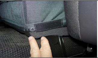
**Step 18. Middle Bottom/MB:** Fold the cover inside out on the sides to keep the Velcro<sup>™</sup> from attaching prematurely to the carpet. Once pulled into down position to the bottom of the seat, line up the cover and press the front hook Velcro<sup>™</sup> to the carpet on the left and right sides.
