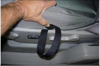
**Step 12. Driver and Passenger Bottoms/DB&PB:** Feed the long outside edge Velcro<sup>™</sup> between the seat and the plastic where shown. Carefully feel under the seat for the Velcro<sup>™</sup> the gap between the seat slide and the seat frame. Pull it tight and connect it to the rear loop Velcro<sup>™</sup> at an angle. The seat slides have grease on them so clean your hands after doing this part.
