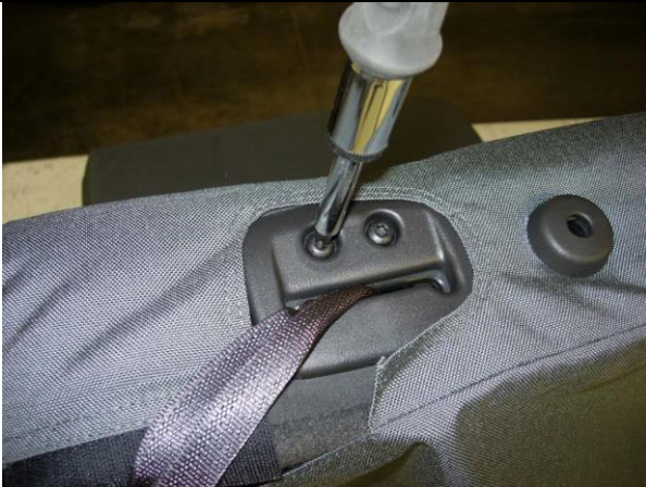
Step 13. Driver & Passenger Top/DT&PT: Temporarily loosen the Phillips screws for the seat belt.
