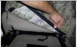
**Step 18. Driver & Passenger Bottoms/DB&PB:** Cloth seat: Pull down and press Velcro<sup>™</sup> to the carpet on the back of the seat. Leather seats: Hook plastic buckle over same metal bar that the plastic hooks are on in Step 17. Pull the Velcro<sup>™</sup> tight thru the buckle and press it together, trim the excess.
