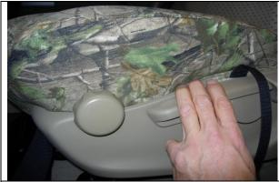
**Step 7. Driver & Passenger Bottoms/DB&PB:** Continue tucking the fabric behind the plastic cowling. Tuck the back edge of the seat cover into the seat, and pull back hard. Line up the seams of the seat cover should to the seams of your seat, they should closely match.
