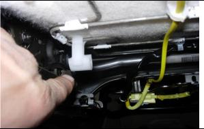
**Step 2. Driver & Passenger Top/DT&PT:** The elastic straps are connected to the seat bottom by the white plastic hooks shown in the photo.
