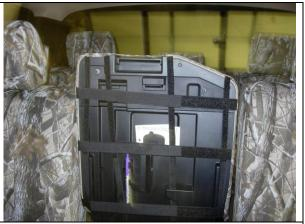
**Step 20. Lid/L:** Connect the Velcro<sup>™</sup> under the lid as shown.
