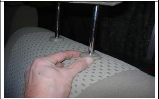
**Step 3. Driver & Passenger Top/DT&PT:** Temporarily remove the headrests by gently lifting up while depressing the push button release as shown. Electric controlled seats: Lift seats up all the way and move forward.
