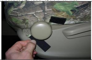
**Step 6. Driver's Bottom with manual controls/DB:** Connect the Velcro<sup>™</sup> under the lumbar knob.
