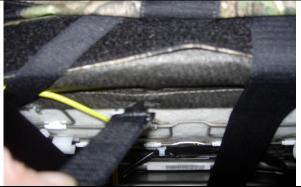
Step 12. Driver & Passenger Bottoms/DB&PB: Clip the (2) short hook Velcro<sup>™</sup> with the buckle sewn to them where shown under the back of the seat, and then connect it to the rear loop Velcro<sup>™</sup>. Trim the excess length of all the Velcro<sup>™</sup>. Some repositioning of the seat cover and Velcro<sup>™</sup> may be needed to provide the best fit. Remember the seams of your seat should closely line up with the seams of the seat cover.
