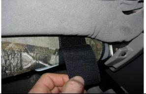
**Step 16. Driver & Passenger Tops/DT&PT:** Route the long hook Velcro<sup>™</sup> under the seat to the metal bar supporting the seats foam 7-8" in from the back edge. Route them over the top of the bar, then back to the loop Velcro<sup>™</sup> sewn inside the seat cover. You may have to smooth and re-fasten more than once.
