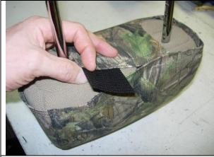
**Step 19. Headrests/H:** Slide the headrest covers on with the extending hook Velcro<sup>™</sup> to the front. Connect them to the loop Velcro<sup>™</sup> sewn inside the back edge.
