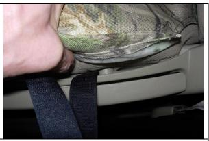
**Step 8. Driver & Passenger Bottoms/DB&PB:** View from the outside edge of the driver seat looking down. Use your fingers to push the seat cushion away from the plastic cowling. Route the long outside edge hook Velcro<sup>™</sup> exactly where shown in front of the plastic nub shown inside the cowling.
