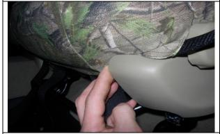
**Step 5. Driver & Passenger Bottoms/DB&PB:** For trucks with electric controls, lift seat up to the ceiling and slide the seats forward all the way. Tuck the fabric behind the plastic cowling in front.
