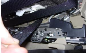
**Step 11. Driver & Passenger Bottoms/DB&PB:** View from behind the driver's underside, next to the center console. Route the inside edge hook Velcro<sup>™</sup> where shown through the gap, just above the metal frame, connecting it to the rear loop Velcro<sup>™</sup>. Route the long hook Velcro<sup>™</sup> under the front of the seat, to the loop Velcro<sup>™</sup> in back, being sure to route them avoiding any seat mechanisms under the seat.
