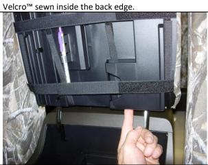
**Step 21. Lid/L:** Feed the Velcro<sup>™</sup> into the hole in the plastic where shown.
