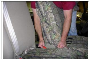
**Step 13. Driver & Passenger Top/DT&PT:** Slide the seat cover on with the extending hook Velcro<sup>™</sup> to the front. Pull the cover down into position as shown, tucking the fabric behind the plastic on the sides. Remember the seams of the seat cover should closely line up with the seams of you seat, so adjust left or right as needed.
