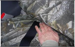
**Step 15. Driver & Passenger Tops/DT&PT:** Tuck the Velcro<sup>™</sup> into the seat. Pull on the fabric not the Velcro<sup>™</sup> from behind the seat while using your other hand in a smoothing action from top to bottom, smoothing and tightening the seat cover.
