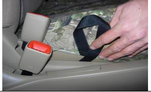
**Step 10. Driver &Passenger Bottoms/DB&PB:** Route the long inside edge hook Velcro<sup>™</sup> where shown between the seat and the plastic cowling.
