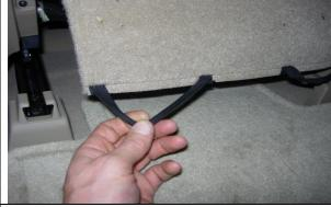
**Step 1. Driver & Passenger Top/DT&PT:** Temporarily remove the elastic straps from the underside of the seat.
