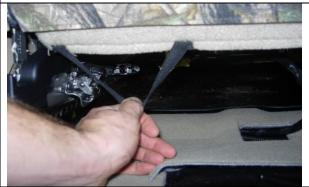
**Step 17. Driver & Passenger Bottoms/DB&PB:** Recline the backrests to their normal position and look at the front side of the seat. You may have to repeat Step 15 and re-tighten the Velcro<sup>™</sup> to remove slack on the front side. Re-connect the elastic straps from the carpeted back panel to the plastic hooks under the seat.
