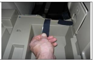
**Step 25. Console/C:** Note the areas where the Velcro<sup>™</sup> will lay inside the console. Clean the areas with rubbing alcohol, scrubbing hard and wiping it dry while it's still wet, don't let it air dry.
