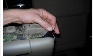
**Step 22. Console/C:** Mate the Velcro<sup>™</sup> behind the seatbelt box and tuck the fabric under the plastic.
