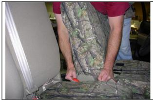
**Step 13. Driver & Passenger Top/DT&PT:** Slide the seat cover on with the extending hook Velcro<sup>™</sup> to the front. Pull the cover down into position as shown, tucking the fabric behind the plastic on the sides. Again, the seams of the seat cover should closely line up with the seams of your seat.
