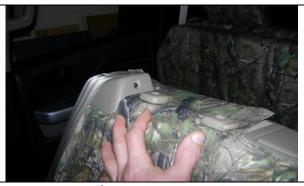
**Step 21. Console/C:** Temporarily remove the headrest by depressing the push button release and gently lifting up. Tuck the fabric of the console cover under the plastic for the headrests and the seatbelt.
