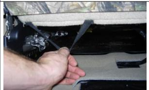
**Step 18. Driver & Passenger Bottoms/DB&PB:** Re-connect the elastic straps from the carpeted back panel to the plastic hooks under the seat.
