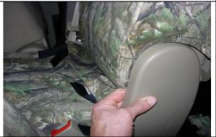
**Step 23. Console/C:** Tuck the bottom left and right sides of the cover in behind the plastic of the hinge area.
