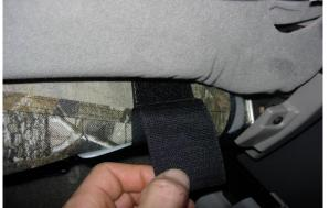
Step 16. Driver & Passenger Tops/DT&PT: Route the long hook Velcro<sup>™</sup> under the seat to the metal bar supporting the seats foam 7-8" in from the back edge. Route them over the top of the bar, then back to the loop Velcro<sup>™</sup> sewn on the seat cover. You may have to smooth and re-fasten more than once.
