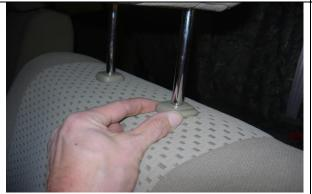
**Step 3. Driver & Passenger Top/DT&PT:** Temporarily remove the headrests by gently lifting up while depressing the push button release as shown.
