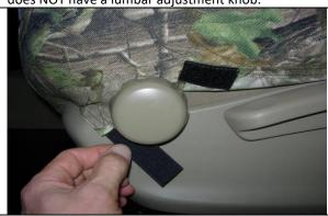
**Step 6. Driver's Bottom/DB:** Connect the Velcro<sup>™</sup> under the lumbar knob.
