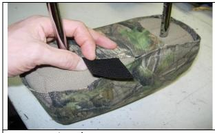
**Step 18. Headrests/H:** Slide the headrest covers on with the extending hook Velcro<sup>™</sup> to the front. Connect them to the loop Velcro<sup>™</sup> sewn inside the back edge.
