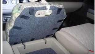
**Step 20. Middle Bottom/MB:** Press the hook Velcro<sup>™</sup> to the carpet on the underside of the seat as shown.
