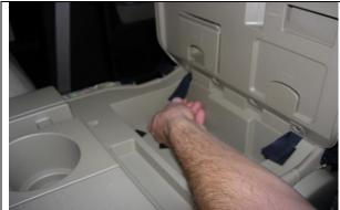
Step 24. Console/C: Open the lid and slide the two rear loop Velcro<sup>™</sup> into the hinge area by lifting the lid up and down, using a sawing motion to slide them in.
