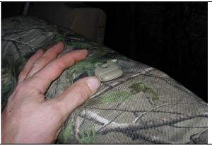
**Step 14. Driver & Passenger Top/DT&PT:** Tuck the fabric of the seat cover under the plastic for the headrests starting with the push button release side first.
