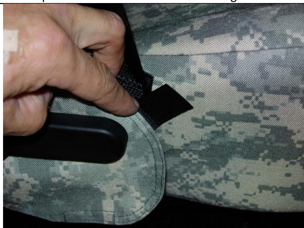
Step 22. Driver & Passenger Tops/DT&PT: Fold this small side hook Velcro™ around the backside and connect it to the carpet on the backside.
