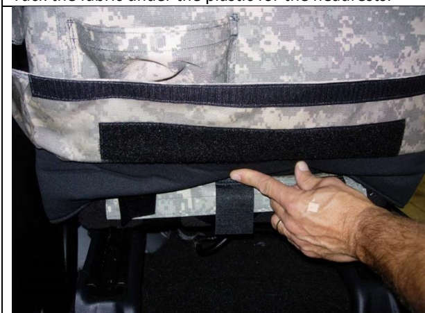
Step 19. Driver & Passenger Tops/DT&PT: Pull the Velcro™ thru to the back.
