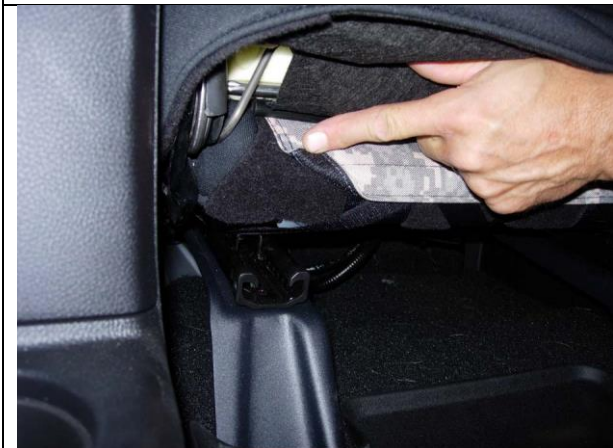
Step 15. Driver & Passenger Bottoms/DB&PB: Pull the back edge of the cover back hard and connect it to the carpet on the back edge of the seat.
