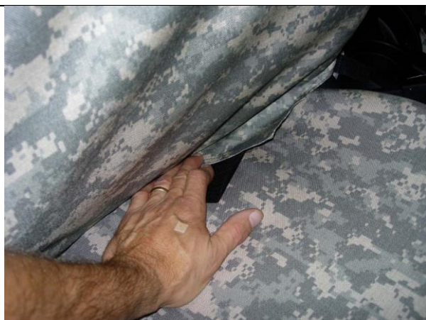
Step 18. Driver & Passenger Tops/DT&PT: Tuck the front edge in.
