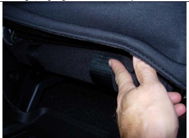
Step 10. Driver & Passenger Bottoms/DB&PB: Connect them to the carpet on the back edge.
