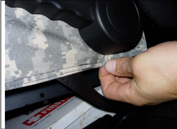
Step 11. Driver Bottom/DB: Connect the Velcro™ under the side lever.
