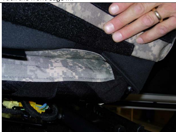
Step 20. Driver & Passenger Tops/DT&PT: Use one hand in a smoothing action down the front of the cover from top to bottom while pulling on the Velcro™ from the back, tuck it under and connect it to the loop Velcro™ sewn inside the back edge.
