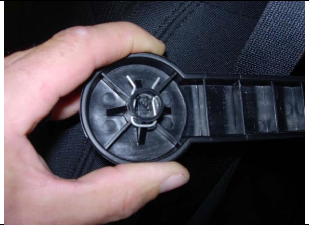
Step 6. Driver & Passenger Top/DT&PT: Slide the pin back over the handle and set it aside.
