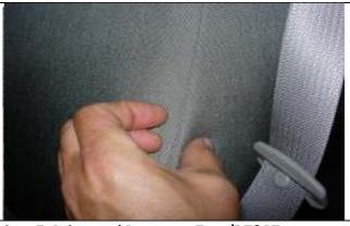
Step 7. Driver and Passenger Tops/DT&PT: Work the material from the seam inside the cover from the main body of the seat cover (fingers) to the middle (thumb). Do this for the front and back of the seat cover top.
