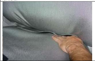
**Step 11. Driver and Passenger Bottoms/DB&PB:** Tuck the back edge of the seat cover into the seat. Pull it into position from behind the seat.
