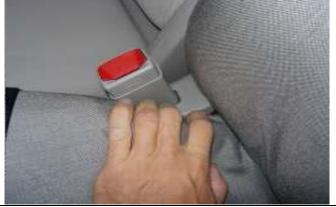
**Step 12. Driver and Passenger Bottoms/DB&PB:** Tuck the seat cover in behind the plastic on the inside back edge.
