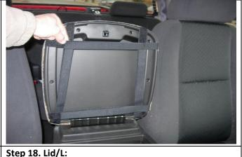
Place the cover on with the lid closed and line up the seams of the cover to the seams of the lid, they should closely match. Connect the Velcro™ under the lid.
