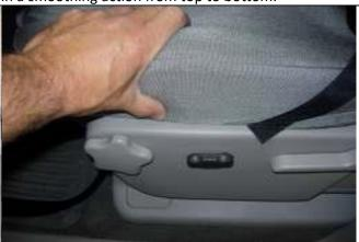
**Step 10. Driver and Passenger Bottoms/DB&PB:** Tuck the seat cover behind the plastic cowling.
