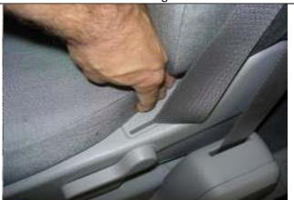
**Step 15. Driver and Passenger Bottoms/DB&PB:** Tuck the seat cover behind the plastic on the outside edge.
