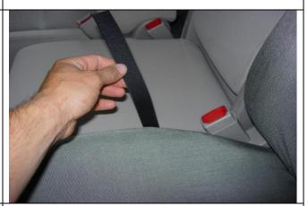
Step 14. Driver and Passenger Bottoms/DB&PB: Tuck the inside long hook Velcro™ down in between the seats. Then, feel for it under the seat, pull it tight and connect it to the rear loop Velcro™ at an angle.
