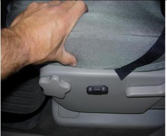
**Step 8. Driver and Passenger Bottoms/DB&PB:** Tuck the seat cover behind the plastic cowling on the outside edge.
