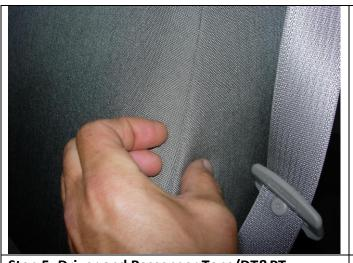
Step 5. Driver and Passenger Tops/DT&PT: Align the seams of the seat cover to the seams of the seat, they should match closely. Work the material from the seam inside the cover from the main body of the seat cover (fingers) to the middle (thumb). Do this for the front and back of the seat
