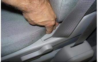
**Step 13. Driver and Passenger Bottoms/DB&PB:** Tuck the seat cover behind the plastic on the outside edge.
