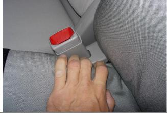
**Step 10. Driver and Passenger Bottoms/DB&PB:** Tuck the seat cover in behind the plastic on the inside back edge. Pull on the back edge of the seat cover.
