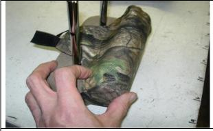
**Step 33. Middle Headrest/MH:** First, slide the cover over the front of the headrest with the extending hook Velcro<sup>™</sup> to the front. Then mate them to the loop Velcro<sup>™</sup> sewn inside the back edge.
