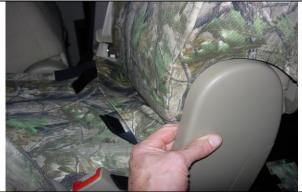
**Step 28. Console/C:** Tuck the bottom left and right sides of the cover in behind the plastic of the hinge area.
