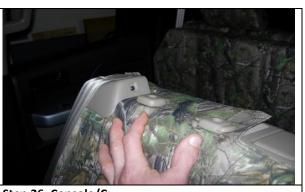
**Step 26. Console/C:** Temporarily remove the headrest by depressing the push button release and gently lifting up. Tuck the fabric of the console cover under the plastic for the headrests and the seatbelt.
