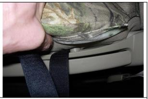
**Step 8. Driver & Passenger Bottoms/DB&PB:** View from the outside edge of the driver seat. Use your fingers to push the seat cushion away from the plastic cowling. Route the long outside edge hook Velcro<sup>™</sup> exactly where shown in front of the plastic nub shown inside the cowling.
