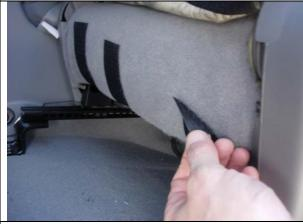
**Step 21. Passenger Bottom/PB:** Install the passenger seat bottom the same as the driver seat bottom, except mate the side and front Velcro to the carpet on the seat.
