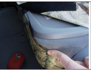
**Step 20.** Passenger Top/PT: Tuck in the left and right front sides, fold the seat flat and pull the back edge up. Mate the Velcro<sup>™</sup> at the back edge,
