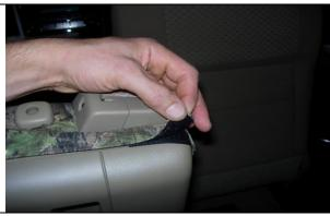
**Step 27. Console/C:** Mate the Velcro<sup>™</sup> behind the seatbelt box and tuck the fabric under the plastic.
