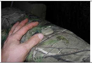
**Step 14. Driver Top/DT:** Tuck the fabric of the seat cover under the plastic for the headrests starting with the push button release side first.
