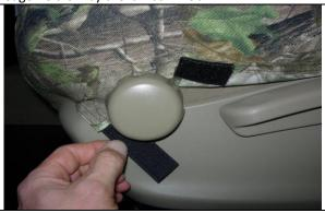
**Step 6. Driver's Bottom/DB:** Connect the Velcro<sup>™</sup> under the lumbar knob, skip this step if no knob exists.
