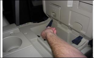
**Step 29. Console/C:** Open the lid and slide the two rear loop Velcro<sup>™</sup> into the hinge area by lifting the lid up and down, using a sawing motion to slide them in.
