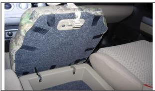
**Step 25. Middle Bottom/MB:** Mate the hook Velcro<sup>™</sup> to the carpet on the underside of the seat as shown.
