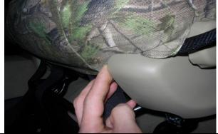
**Step 5. Driver & Passenger Bottoms/DB&PB:** If you have electric seats be sure to lift the seat up as high as it will go. This will pull everything away from your seat and free up some space. Tuck the fabric behind the plastic cowling in front.
