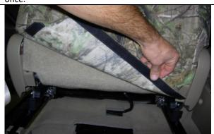
**Step 18. Driver Top /DT:** Lastly, connect the hook Velcro<sup>™</sup> to the carpeted flap, starting on the inside next to the center console, working your way out.
