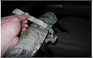
**Step 24. Middle Bottom/MB:** Tilt the seat bottom up and feed the release strap through the provided opening in back.
