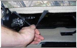
**Step 17. Driver Top/DT:** Re-connect the elastic straps from the carpeted back panel to the plastic hooks under the seat.
