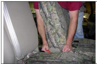
**Step 13. Driver & Passenger Top/DT&PT:** Slide the seat cover on with the extending hook Velcro<sup>™</sup> to the front. Pull the cover down into position as shown, tucking the fabric behind the plastic on the sides. The seams of the seat cover should closely line up with the seams of your seat.
