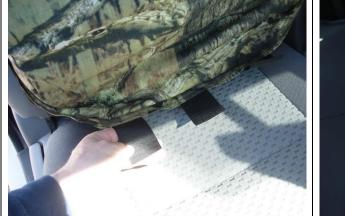
**Step 19. Passenger Top/PT:** Place the cover on with the extending hook Velcro<sup>™</sup> to the front, and tuck the fabric under the headrest plastic.
