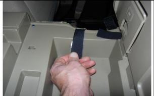
**Step 30. Console/C:** Note the areas where the Velcro<sup>™</sup> will lay inside the console. Clean the areas with rubbing alcohol, scrubbing hard and wiping it dry while it's still wet, don't let it air dry.
