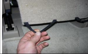
**Step 1. Driver/DT:** Temporarily remove the elastic straps from the underside of the seat.
