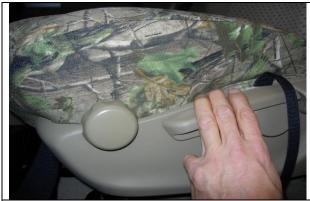
**Step 7. Driver & Passenger Bottoms/DB&PB:** Continue tucking the fabric behind the plastic cowling. Tuck the back edge of the seat cover into the seat. Line up the seams of the seat cover should to the seams of your seat, they should closely match.
