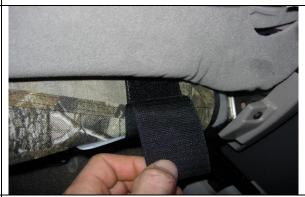
**Step 16. Driver Top/DT:** Route the long hook Velcro<sup>™</sup> under the seat to the metal bar supporting the seats foam 7-8" in from the back edge. Route them over the top of the bar, then back to the loop Velcro<sup>™</sup> sewn inside the seat cover. You may have to smooth and re-fasten more than once.
