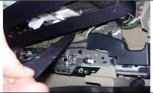
**Step 11. Driver & Passenger Bottoms/DB&PB:** View from behind the driver's underside, next to the center console. Route the inside edge hook Velcro<sup>™</sup> where shown through the gap, just above the metal frame, mating it to the rear loop Velcro<sup>™</sup>. Route the long hook Velcro<sup>™</sup> under the front of the seat, to the loop Velcro<sup>™</sup> in back, being sure to route them avoiding any seat mechanisms under the seat.
