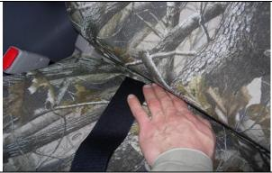
Step 15. Driver/DT: Tuck the Velcro<sup>™</sup> into the seat. Pull on the fabric not the Velcro<sup>™</sup> from behind the seat while using your other hand in a smoothing action from top to bottom, smoothing and tightening the seat cover.
