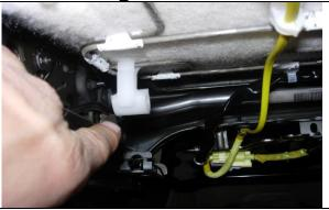
**Step 2. Driver Top/DT:** The elastic straps are connected to the seat bottom by the white plastic hooks shown in the photo.
