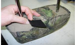
**Step 23. Headrests/H:** Slide the headrest covers on with the extending hook Velcro<sup>™</sup> to the front. Mate them to the loop Velcro<sup>™</sup> sewn inside the back edge.
