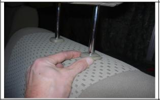
**Step 3. Driver & Passenger Top/DT&PT:** Temporarily remove the headrests by gently lifting up while depressing the push button release as shown.
