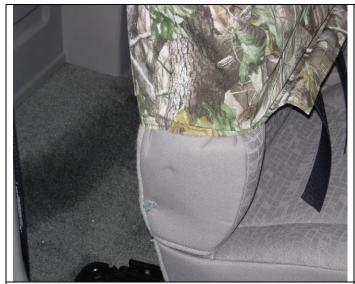
**Step 1. Driver & Passenger tops/DT&PT:** Temporarily remove the side lever attached to the backrest with a Torx # 15.
