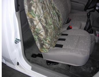
**Step 2. Driver & Passenger tops/DT&PT:** Position the cover so the seams of the seat cover closely line up with the seams of the seat. Tuck the hook Velcro<sup>™</sup> into the seat and mate the hook to the loop Velcro<sup>™</sup> sewn inside the back edge. Be careful to not over tighten the hook Velcro<sup>™</sup> because they permanently dent your seat.
