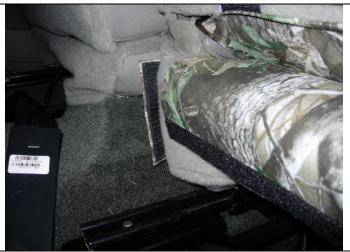
**Step 4. Driver and Passenger bottom/DB&PB:** View from behind the passenger seat. Line up the seat cover seams with the seams on the seat, they should closely match. Pull the inside flap of seat cover behind the seat belt back and press the Velcro<sup>™</sup> to the carpet on the seat. Tuck the rear part of the seat cover into the seat, pull it down to the bottom edge and connect it to the carpet on the seat.
