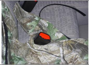
**Step 3. Passenger bottom/PB:** Place the seat cover on with the long hook Velcro<sup>™</sup> to the front. Feed the female part of the seat belt though the provided opening as shown and tuck the material flap behind the seat belt around to the back of the seat.
