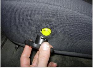
Next, temporarily remove the lumbar knob from the driver's side by gently wiggling it off, either up and down, or side to side. Remove the plastic drink holders on the front of the seat by lifting up the plastic release under the front, and sliding the unit forward.
