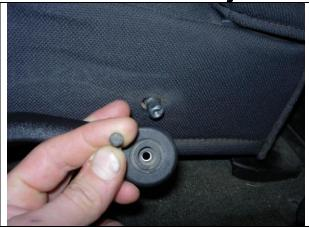
Temporarily remove the recline and access lever from the driver and passenger seats using a Torx 20 bit. All of the parts of the seat cover are labeled inside. Use the seat cover Piece Identification Chart to ID the different parts of the seat cover.
