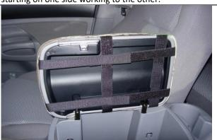
**Step 14. Lid/L:** Carefully detach the Velcro<sup>™</sup> and place the lid cover on with the lid down. Open the lid and connect the Velcro<sup>™</sup> on the underside as shown.
