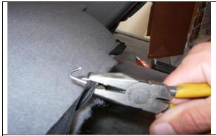
**Step 11. Driver and Passenger Top/DT&PT:** Using pliers, clamp the provided metal hooks to the elastic straps with the hook up. Connect the hooks under the seat to the metal bar.
