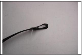
**Step 6. Driver and Passenger Bottom/DB&PB**: Clip the hooks of this hook Velcro<sup>™</sup> under the back edge of the seat to the metal bar that the hog rings or plastic clips were fastened to. Press it to the loop Velcro<sup>™</sup> on the back of the seat cover bottom. This will keep the seat cover from shifting around. Use two straps for each seat bottom.
