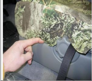
**Step 3. Driver and Passenger Bottom/DB&PB**: Tuck the fabric behind the plastic on the outside edge.
