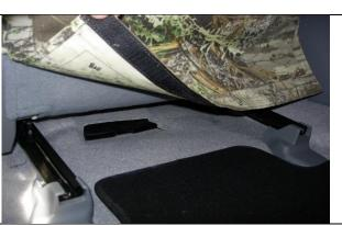
**Step 12. Driver and Passenger Top/DT&PT:** Pull the back of the seat cover down and press the hook Velcro<sup>™</sup> to the carpet on the back edge of the backrest, starting on one side working to the other.
