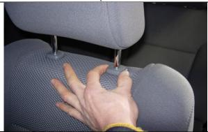
**Step 7. Driver and Passenger Top/DT&PT:** Temporarily remove the headrests by depressing the push button release and gently lifting up in the middle.
