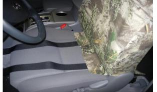
**Step 8. Driver and Passenger Top/DT&PT:** Slide the seat covers on with the long hook (sticky) Velcro<sup>™</sup> to the front.
