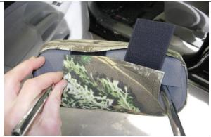
**Step 13. Headrests/H**: Slide the headrest covers with the extending hook Velcro<sup>™</sup> to the front, connecting the Velcro<sup>™</sup> in back as shown.
