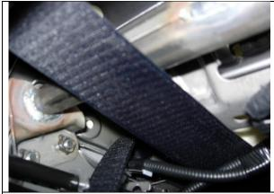
**Step 5. Driver and Passenger Bottom/DB&PB**: Carefully feel under the seat for the Velcro<sup>™</sup>, it will be in a gap between the seat slide and the main frame of the seat. Route it at an angle and connect it to the loop Velcro<sup>™</sup> sewn on the back edge. Route the inside edge Velcro<sup>™</sup> the same way, between the plastic and the seat, through the gap above the seat slide, and then connect it to the loop Velcro<sup>™</sup> on the back.
